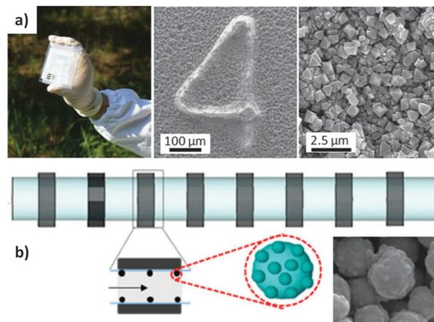
Fig. 39 (a) Sunlight driven photolithography of a Cu plated plastic board for the subsequent HKUST-1 film growth (insets), from Okada *et al.*<sup>172</sup> (b) schematic of the microfluidic device used for the flow reaction using  $\text{Fe}_3\text{O}_4@ZIF-8$  magnetic framework composite (inset), from Faustini *et al.*<sup>216</sup>
