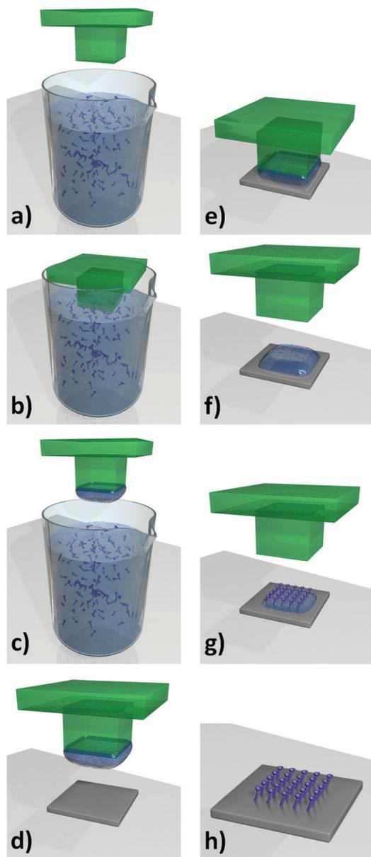
Fig. 4 Surface functionalisation by microcontact printing ( $\mu$ CP). (a–c) A lithographed stamp is inked with solution containing the functional units. (d–f) The solution is then transferred to the substrate by placing the stamp in contact with the substrate. (g and h) The solvent is then allowed to evaporate, producing the self-assembled monolayer (SAM). Video animation provided as ESI.†
