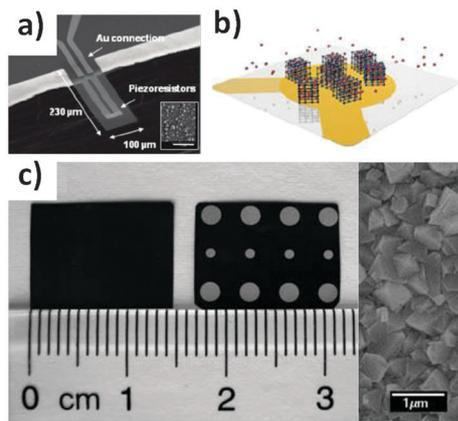
Fig. 31 (a) SEM of piezoresistive microcantilever and inset SEM of MOF deposition (scale bar 2  $\mu\text{m}$ ), from Allendorf *et al.*,<sup>264</sup> (b) schematic of the QCM platform (transparent plate) where MOFs are deposited on the gold electrodes (yellow), from Tsotsalas,<sup>55</sup> (c) photograph of HKUST-1 MOF film (left) with Al electrodes attached (right) and SEM image of MOF film surface, from Liu *et al.*<sup>266</sup>
