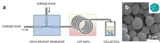
Fig. 26 Microfluidic production and immobilization of  $\text{Fe}_3\text{O}_4@ZIF-8$ . (a) Schematic of the device used; (b) SEM images of magnetic iron oxide nanoparticles successfully coated with ZIF-8 MOF. From Faustini *et al.*<sup>150</sup>
