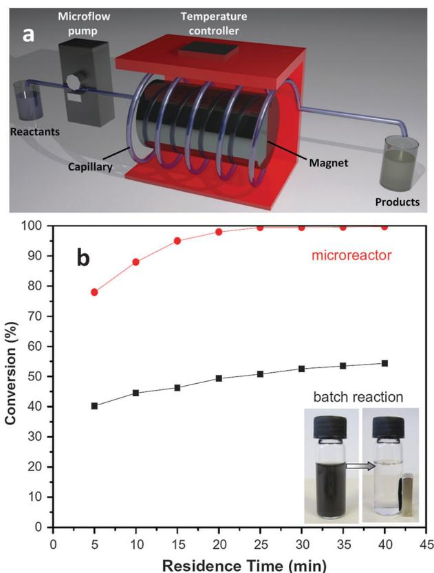
Fig. 25 (a) Schematic of the reactor used for the condensation reaction between benzaldehyde and ethyl cyanoacetate using Fe<sub>3</sub>O<sub>4</sub>@ZIF-8 MFC immobilized along the tube with a magnet; (b) results of the catalytic conversion. The inset shows the fast collection of the composite with an external magnet. From Zhang *et al.*<sup>216</sup>
