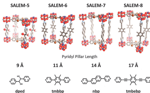
Fig. 2 Increasing pore sizes in an isorecticular series of pillared-paddlewheel MOFs synthesized via SALE. The value in Å represents the length of the dipyrindyl linkers utilized for SALE on the parent MOF SALEM-5 .
