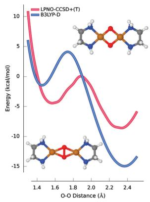
Fig. 2 The most accurately calculated PES and the corresponding one calculated with B3LYP-D, ZORA and COSMO corrections using the def2-TZVP basis set. The peroxo and bis- $(\mu$ -oxo) structures of  $[Cu_2(en)_2(O)_2]^{2+}$ . Adapted with permission from D. G. Liakos and F. Neese, *J. Chem. Theory Comput.*, 2011, **7**, 1511–1523. Copyright 2011 American Chemical Society.
