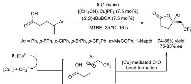
Scheme 22 Copper-catalyzed enantioselective oxotrifluoromethylation of unactivated olefins.
