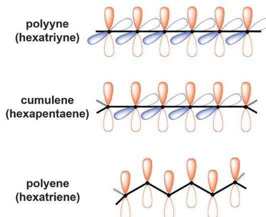
Fig. 5 Schematic depiction of  $\pi$ -orbitals of structures with six  $\pi$ -electrons in the longest conjugated segment shown in red: a polyne, cumulene, and polyene. The orthogonal and degenerate six- $\pi$ -electron segment of the hexatriyne and the orthogonal four- $\pi$ -electron segment of the [5]cumulene are shown in blue.
