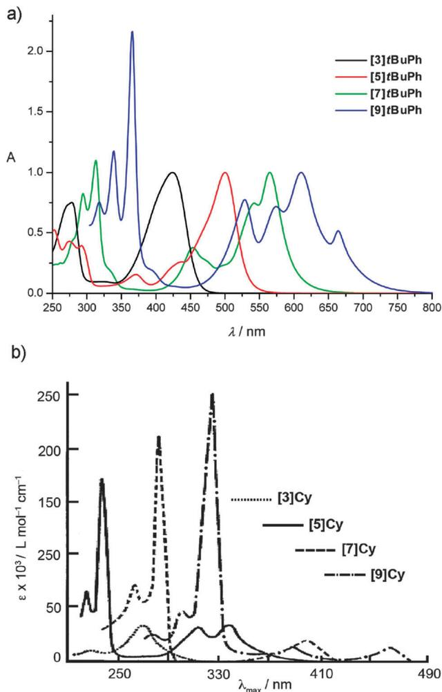
Fig. 4 UV/vis spectra of  $[n]$ cumulenes. (a)  $[n]$ tBuPh measured in Et<sub>2</sub>O; spectra normalized to the most intense low energy absorption and (b)  $[n]$ Cy measured in Et<sub>2</sub>O (adapted with permission from ref. 135. Copyright 1964 John Wiley & Sons).
