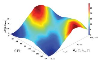
Fig. 9 Computed potential energy surface of truncated 13-Me (BLYP35/ COSMO(CH<sub>2</sub>Cl<sub>2</sub>) level). <sup>219</sup>  $\Omega$  represents the dihedral angle for the redox centres and  $\Theta_{\mathrm{eff}}$  for the bridge rotation. Adapted with permission from M. Parthey, J. B. G. Gluyas, M. A. Fox, P. J. Low and M. Kaupp, Chem. -Eur. J., DOI: 10.1002/chem.201304947. Copyright @ 2014 WILEY-VCH Verlag GmbH & Co. KGaA, Weinheim.
