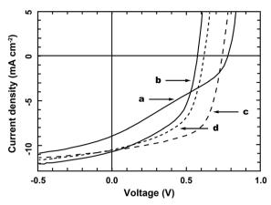
Fig. 26 Current density vs. voltage (J-V) curves under 100 mW cm<sup>-2</sup> air mass 1.5G simulated solar illumination, of (a) ITO/MoO<sub>3</sub>/286:C<sub>60</sub> (105 °C)/ C<sub>60</sub>/BCP/Ag; (b) ITO/MoO<sub>3</sub>/FDTS/**286**:C<sub>60</sub> (105 °C)/C<sub>60</sub>/BCP/Ag; (c) ITO/  $MoO_3/286$  (105 °C)/C<sub>60</sub>/BCP/Ag; and (d) ITO/MoO<sub>3</sub>/FDTS/286 (105 °C)/ C<sub>60</sub>/BCP/Ag. (Reproduced with permission from ref. 144. Copyright 2010.
