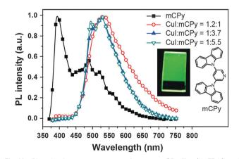
Fig. 11 Photoluminescence spectra of a neat mCPy film (at 77 K) and Cul:mCPy films with different ratios at room temperature under excitation at 350 nm (inset: photographic image of a Cul:mCPy film excited at 365 nm using a UV lamp). (Reproduced with permission from ref. 62. Copyright 2011, American Chemical Society.)
