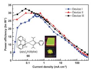
**Fig. 9** Power efficiency vs. current density curves of PHOLEDs using **98** as phosphor (inset: photographs showing phosphorescent emission of **98** in its film and powder states). (Reproduced with permission from ref. 51. Copyright 2009, Royal Society of Chemistry.)
