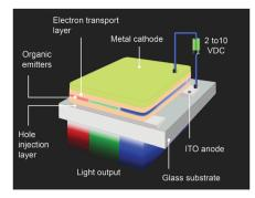
Fig. 4 Device structures of prototype sandwich-structured OLEDs.
