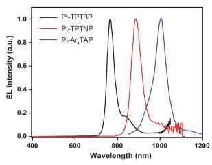
Fig. 13 Electroluminescence spectra of PHOLEDs using 238, 245 and 246 as the emitter, respectively, in the PVK:PBD host matrix. The bathochromic shifts in emission from 750 to 1000 nm are due to conjugation extension from phenyl to naphthyl to anthryl in their porphyrin rings. (Reproduced with permission from ref. 96. Copyright 2011, American Chemical Society.)
