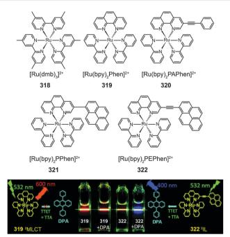
Fig. 30 Molecular structures of Ru(II) sensitizers 318-322 and photographic images of upconversion emissions by 319 and 322. (Reproduced with permission from ref. 188. Copyright 2011, Wiley-VCH Verlag GmbH &
