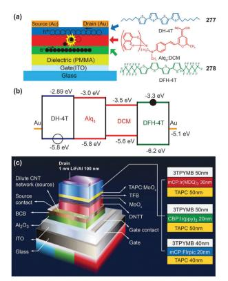
Fig. 21 (a and b) Device configuration and energy level scheme of a trilayer OLET using Alg<sub>3</sub>:DCM, DH-4T and DFH-4T as emitting, holetransporting, and electron-transporting layers, respectively. (c) Device structures of a trilayer OLET with direct integration of red, green and blue OLED and OTFT. (Reproduced with permission from ref. 8 and 121. Copyright 2011 and 2010, respectively, American Association for the Advancement of Science and Nature Publishing Group.)
