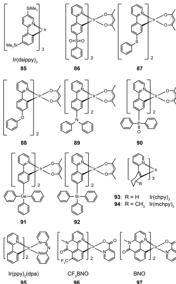
Notably, **96** and **97** are solution processible. The phosphorescent organic light-emitting diode (PHOLED) obtained from the spin-coated complex **96** emits blue-green color with a high current efficiency of 89.1 cd A<sup>-1</sup> (69.8 lm W<sup>-1</sup>) at 100 cd m<sup>-2</sup>.
