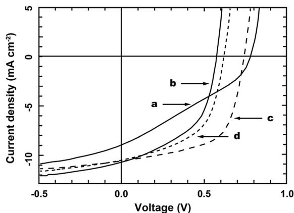
Fig. 26 Current density vs. voltage ( $J$ - $V$ ) curves under  $100 \text{ mW cm}^{-2}$  air mass 1.5G simulated solar illumination, of (a) ITO/MoO<sub>3</sub>/286:C<sub>60</sub> (105 °C)/C<sub>60</sub>/BCP/Ag; (b) ITO/MoO<sub>3</sub>/FDTS/286:C<sub>60</sub> (105 °C)/C<sub>60</sub>/BCP/Ag; (c) ITO/MoO<sub>3</sub>/286 (105 °C)/C<sub>60</sub>/BCP/Ag; and (d) ITO/MoO<sub>3</sub>/FDTS/286 (105 °C)/C<sub>60</sub>/BCP/Ag. (Reproduced with permission from ref. 144. Copyright 2010, Elsevier B.V.)
