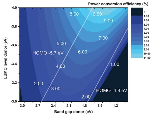
Fig. 24 Theoretical relations between the power conversion efficiency and the HOMO level of the donors in PCBM-based bulk OPVs. (Reproduced with permission from ref. 129. Copyright 2006, Wiley-VCH Verlag GmbH & Co. KGaA.)
