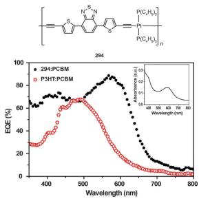
Fig. 27 Absorption wavelength-dependent external quantum efficiencies of an OPV device containing Pt(II)-based organometallic D-A conjugated polymers (inset: absorption spectra of 294). (Reproduced with permission from ref. 6. Copyright 2007, Nature Publishing Group.)
