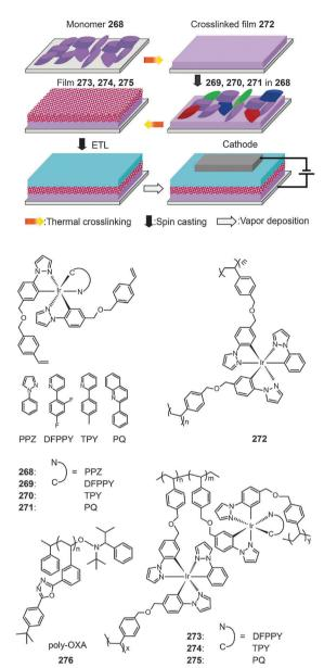
Fig. 18 procedure of solution-processed multi-layer devices on the basis of crosslinkable monomers 268-271 and the corresponding crosslinked polymers **272–275**. (Reproduced with permission from ref. 116. Copyright 2009, Wiley-VCH Verlag GmbH & Co. KGaA.)
