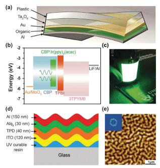
Fig. 19 (a) Device configuration of a PHOLED using Ta<sub>2</sub>O<sub>5</sub> as the light out-coupling layer. (b) The energy level diagram of active layers used in PHOLEDs. (c) The photographic image of the device in operation. (d) A quasi-periodic buckling structure designed for enhancing light outcoupling. (e) Topographic AFM image of buckling patterns formed by a 10 nm-thick aluminium layer. (Reproduced with permission from ref. 117a and b. Copyright 2011 and 2010, Nature Publishing Group.)
