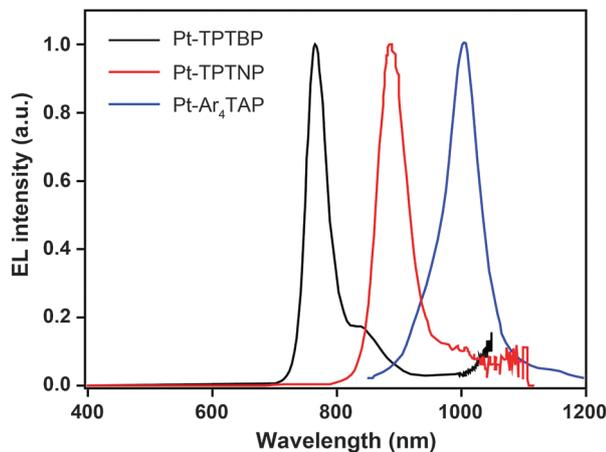
**Fig. 13** Electroluminescence spectra of PHOLEDs using **238**, **245** and **246** as the emitter, respectively, in the PVK:PBD host matrix. The bathochromic shifts in emission from 750 to 1000 nm are due to conjugation extension from phenyl to naphthyl to anthryl in their porphyrin rings. (Reproduced with permission from ref. 96. Copyright 2011, American Chemical Society.)
