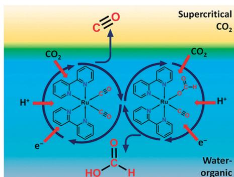
Fig. 4 Representation of a biphasic reaction medium with a supercritical CO<sub>2</sub> phase and liquid water-organic phase for homogeneous CO<sub>2</sub> reduction. Reproduced with permission from ref. 22. Copyright 2013, American Chemical Society.
