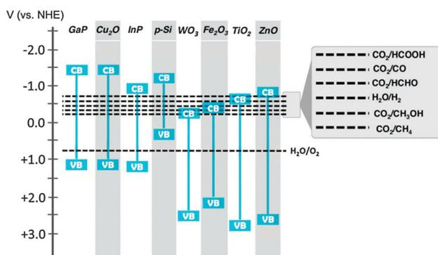
Fig. 5 Band gap energies of selected semiconductor materials and redox potentials of water oxidation and CO<sub>2</sub> reduction reactions.
