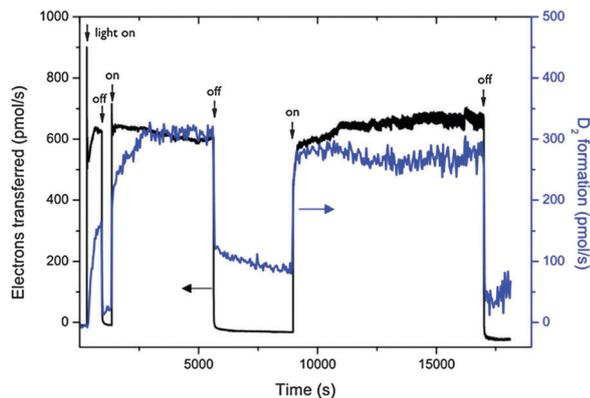
Fig. 17 Monitoring of photocurrent and D<sub>2</sub> formation out of deuterated water in a fuel cell type solar membrane PEC cell with interrupted illumination. Reproduced from ref. 24 with permission from the PCCP owner societies.
