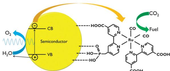
Fig. 8 Representation of CO<sub>2</sub> reduction using a polypyridyl catalyst anchored to a semiconductor surface. In this scheme, both carboxylic and phosphonic acid linking groups are shown.
