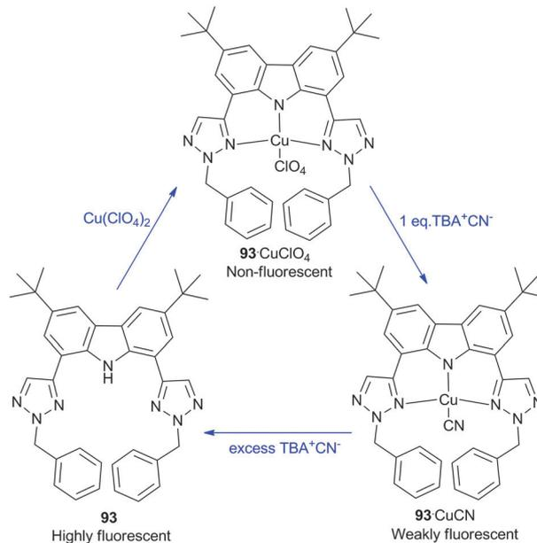
Scheme 9 The proposed mechanism of CN<sup>-</sup> sensing by the **93**-Cu(II) complex.
