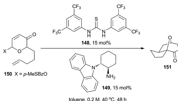
Scheme 20 Oxidopyrylium cycloaddition catalysed by **148** and **149**.
