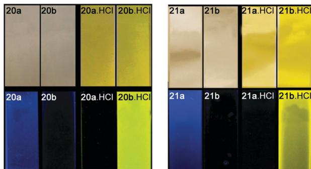
Fig. 4 Colourless solutions of neutral compounds in  $\text{CHCl}_3$  turn yellow upon protonation (top); fluorescence (excitation 365 nm) is quenched in electron-rich compounds **20a**, **21a** and is 'turned on' in electron poor compounds **20b**, **21b** (bottom). Reproduced with permission from *Chem. Commun.* 2011, **47**, 5539–5541 © Royal Society of Chemistry.
