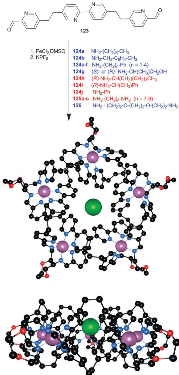
Fig. 22 (top) Self-assembly of a pentafoil knot from aldehyde **123**, FeCl<sub>2</sub> and amines **124**–**126**. The amines capable of forming a pentafoil knot are shown in blue, with the other amines in red. (below) Two views of the crystal structure of the knot formed between **123** and **126**; hydrogen atoms, counterions and solvent molecules are omitted for clarity; chloride and iron(II) ions are shown in spacefill with the rest of the knot shown in ball-and-stick.
