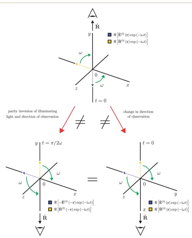
Fig. 4 A parity inversion of the lin  $\perp$  lin illuminating light and the direction of observation  $\hat{\bf R}=\hat{\bf y}$  through the origin can be mimicked in the z=0 plane by leaving the light unaltered and changing the direction of observation from  $\hat{\bf R}=\hat{\bf y}$  to  $\hat{\bf R}=\hat{\bf x}$ .
