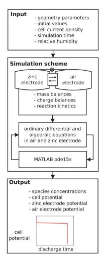
**Fig. 3** Flowchart of the conducted simulations for the investigated ZA13 button cell type battery with model input and output variables indicated. Computation time with this model approach is in the range of ten seconds (using a standard quad-core office computer).
