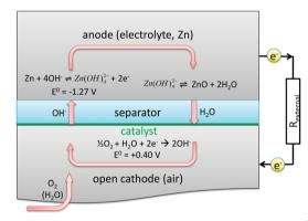
Fig. 1 Sketch of reactions in a zinc air battery during discharging.<sup>1</sup>
