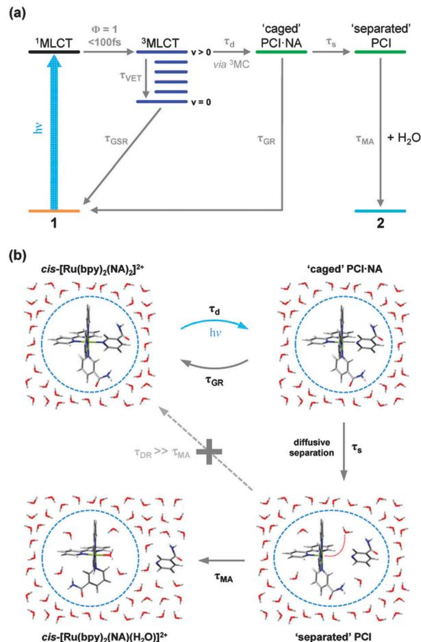
Fig. 6 (a) Kinetic scheme illustrating the *major* pathways and associated time constants ( $\tau$ ), used to model the photodissociation dynamics of **1** in  $\text{H}_2\text{O}$ . The individual steps involved in this kinetic scheme are discussed further in the main text (Section 3.3). (b) Pictorial schematic of the post-dissociation processes involving the PCI and formation of the photoproduct **2**.
