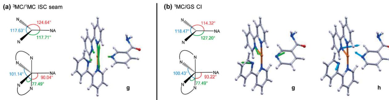
Fig. 9 (a) MECP of the CASSCF calculated <sup>3</sup>MC/<sup>1</sup>MC ISC seam. Equatorial and axial angles of this geometry as well as the gradient difference motion (**g**) are presented. (b) MECP of the CASSCF calculated <sup>1</sup>MC/GS CI, of quasi-JT type, and branching space. Equatorial and axial angles of this geometry as well as the gradient difference (**g**) and derivative coupling motions (**h**) are presented.
