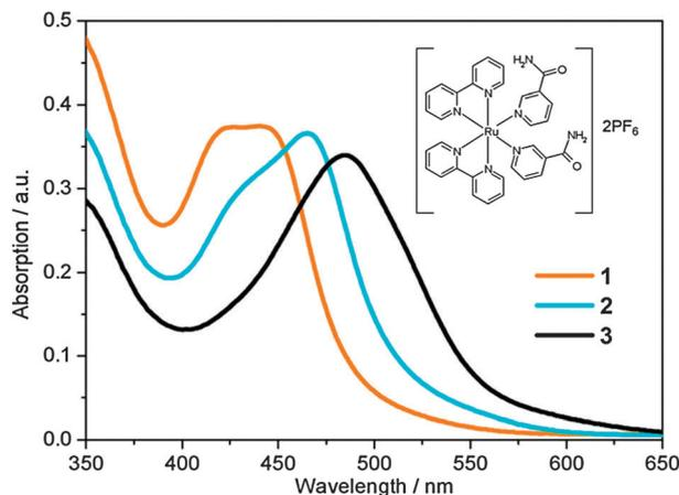
Fig. 1 Static UV/Vis absorption spectra of  $[\text{Ru}(\text{bpy})_2(\text{NA})_2]^{2+}$  (**1**, orange),  $[\text{Ru}(\text{bpy})_2(\text{NA})(\text{H}_2\text{O})]^{2+}$  (**2**, cyan) and  $[\text{Ru}(\text{bpy})_2(\text{H}_2\text{O})_2]^{2+}$  (**3**, black). Irradiation of **1** with 465 nm for 50 s yields **2**. Further irradiation of **2** for 1 h 50 min yields **3**. Molecular structure of **1** is shown inset.
