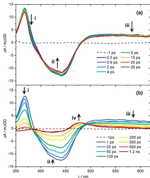
**Fig. 3** UV/Vis TAS of 890  $\mu\text{M}$  aqueous solution of **1** over pump-probe delay ranges (a)  $t = -1$  to 25 ps and (b)  $t = -1$  ps to 1.2 ns, following photoexcitation at 340 nm. Growth/decay features i–iv highlighted indicate the spectral location assigned to the  $^3\text{MLCT}$  ESA, GSB of **1**, absorption of the PCI and, finally, photoproduct **2**, respectively. See main text for further details.
