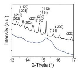
Fig. 6 Synchrotron-based XRD data ( $\lambda=0.08856$  nm) obtained at the end of the 5th discharge (blue line) and charge (black line) cycles. Peaks for monoclinic β-sulfur are indexed. The different full width at half maximum intensities indicate anisotropic crystal growth. The fact that the peak at a  $2\theta$  of  $\sim15.5^\circ$  (blue line) is much broader than those of β-sulfur is due to the lower degree of crystallinity of the Li<sub>2</sub>S.
