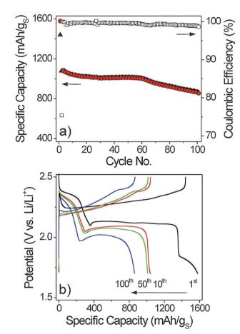
Fig. 2 Cycling performance of the Li-S cells at 25 °C. The 1st cycle was performed at C/50. Thereafter, discharge and charge current rates of C/5 and C/8, respectively, were used. (a) Specific capacity and coulombic efficiency versus cycle number. The charge and discharge capacities are shown as black triangles and red circles, respectively. (b) Voltage-capacity curves for the 1st (black), 10th (red), 50th (green) and 100th (blue) cycles.
