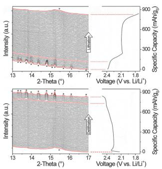
Fig. 5 Synchrotron-based in operando XRD data ( $\lambda$  = 0.08856 nm) obtained on a Li–S pouch cell cycled at C/5 (5th cycle). Cubic Li<sub>2</sub>S and monoclinic  $\beta$ -sulfur indicated by the plus and asterisk marks, respectively, can be clearly observed. The corresponding voltage profiles are shown on the right.
