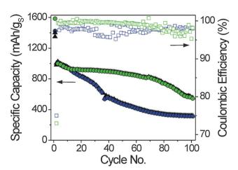
**Fig. 3** Cycling performance of the Li–S cells at 40 °C (green) and 60 °C (blue). After the formation cycle at C/50, the discharge and charge current rates were increased to C/5 and C/8, respectively. Both the specific charge (black triangles) and discharge (colored circles) capacities and the coulombic efficiencies are shown.
