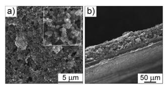
(a) Top view and cross-sectional (b) SEM images of a noncalendered,  $\sim 45 \ \mu m$ -thick sulfur cathode on primed aluminum before galvanostatic cycling, showing the electrode is porous and the top surface is largely crack-free on the micrometer-length scale. The side length of the high-magnification image in the inset of panel (a) is 1.1 µm.
