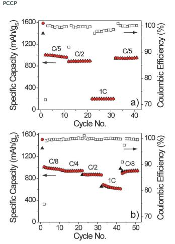
Fig. 4 Specific charge (black triangles) and discharge (red circles) capacities and coulombic efficiency *versus* cycle number for different C-rates. (a) The discharge current was increased from C/5 to 1C while maintaining the charge current rate at C/8. (b) The charge current was increased from C/8 to 1C while keeping the discharge current rate constant at C/5. Note that the rate performance was measured after 1 cycle at C/50 was completed.
