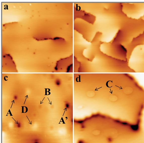
Fig. 1 STM topographic images of two 30 ML thick CaO films annealed to (a) 1200 K and (b) 1000 K ( $500 \times 500 \text{ \AA}^2$ ). Note the different defect concentrations. (c and d) High resolution images showing the four different defect types discussed in the text ( $200 \times 200 \text{ \AA}^2$ ).
