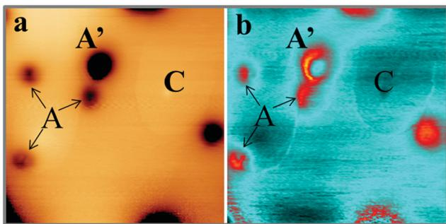
Fig. 3 (a) STM topographic and (b) corresponding  $dI/dV$  image of a 30 ML thick CaO film. Note the spatial proximity between the A and C defects. The latter is best seen in the conductance image due to its small apparent height ( $200 \times 200 \text{ \AA}^2$ ).
