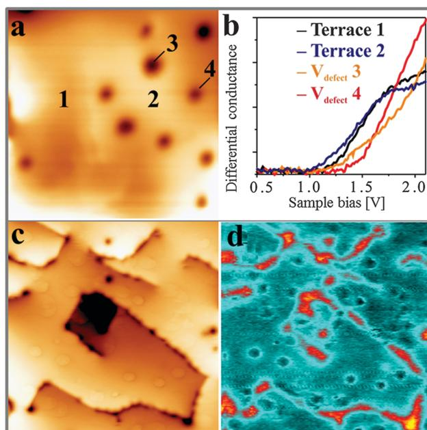
Fig. 6 (a) STM topographic image of a 15 ML  $\text{CaO}_{\text{Mo}}$  film ( $200 \times 200 \text{ \AA}^2$ ) and (b)  $dI/dV$  spectra taken at the indicated surface positions. The setpoint bias was set to 2.0 V in all four cases. (c and d) Topographic image and corresponding  $dI/dV$  map taken at 3.5 V on a 30 ML thick  $\text{CaO}_{\text{Mo}}$  film ( $450 \times 450 \text{ \AA}^2$ ). The most prominent defects in the image are the Mo dopants (C-defects) and the dislocation lines.
