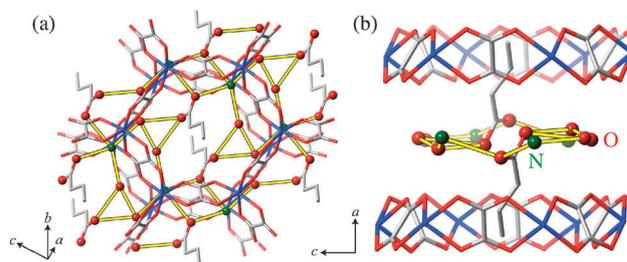
Fig. 11 Possible hydrogen-bond arrangements in  $(\text{NH}_4)_2(\text{adp})[\text{Zn}_2(\text{ox})_3] \cdot 3\text{H}_2\text{O}$ . Yellow thick lines represent hydrogen bonds whose length is shorter than 3.1 Å. (a) Perspective view along the  $a$ -axis. (b) Perspective view along the  $b$ -axis.
