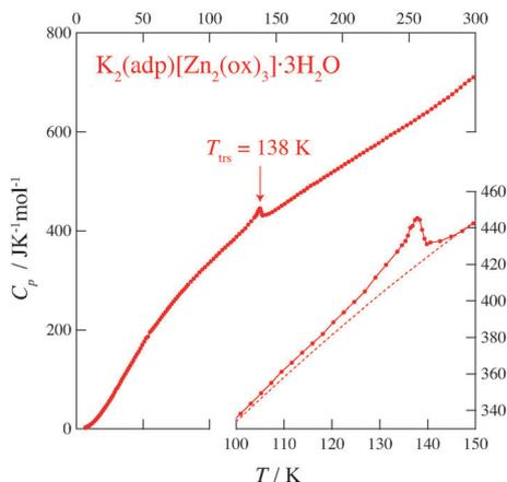
Fig. 3 Heat capacity of  $\text{K}_2(\text{adp})[\text{Zn}_2(\text{ox})_3]\cdot 3\text{H}_2\text{O}$ . The inset shows an enlarged plot around the phase transition. The dashed line represents the baseline for the transition. See text for the details.
