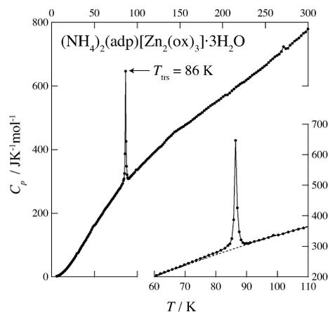
Fig. 2 Heat capacity of  $(\text{NH}_4)_2(\text{adp})[\text{Zn}_2(\text{ox})_3]\cdot 3\text{H}_2\text{O}$ . The inset shows an enlarged plot around the phase transition. The dashed line represents the baseline for the transition. See text for the details.
