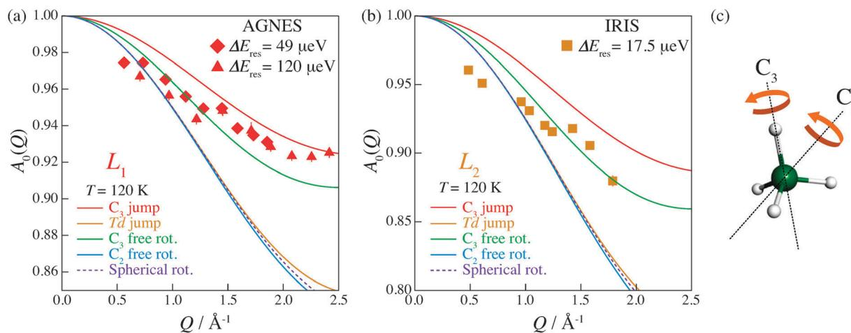
**Fig. 10** Elastic incoherent structure factor (EISF) of  $(\text{NH}_4)_2(\text{adp})[\text{Zn}_2(\text{ox})_3]\cdot 3\text{H}_2\text{O}$  for (a) the  $L_1$  mode measured by AGNES and (b) the  $L_2$  mode measured by IRIS. Solid curves represent the calculated EISF based on several model functions. See text for the details. (c) Structure of ammonium ions composed of four hydrogen atoms (white) and a nitrogen atom (green). The twofold ( $C_2$ ) and threefold ( $C_3$ ) axes are exhibited.
