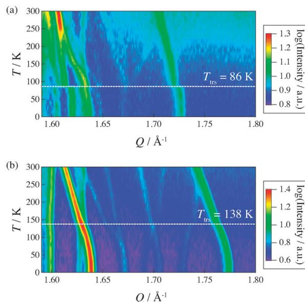
Fig. 5 Two-dimensional intensity maps obtained by neutron powder diffraction on IRIS for (a)  $(\text{NH}_4)_2(\text{adp})[\text{Zn}_2(\text{ox})_3]\cdot 3\text{H}_2\text{O}$  and (b)  $\text{K}_2(\text{adp})[\text{Zn}_2(\text{ox})_3]\cdot 3\text{H}_2\text{O}$ . The intensity is given on a logarithmic scale. The white dashed line represents each transition temperature.
