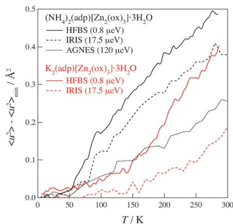
Fig. 6 Mean square displacements of  $(\text{NH}_4)_2(\text{adp})[\text{Zn}_2(\text{ox})_3] \cdot 3\text{H}_2\text{O}$  (black line) and  $\text{K}_2(\text{adp})[\text{Zn}_2(\text{ox})_3] \cdot 3\text{H}_2\text{O}$  (red line) as functions of temperature. The number in the parenthesis denotes the energy resolution of each instrument. The solid, dashed, and dotted lines correspond to the data taken on HFBS, IRIS, and AGNES, respectively.
