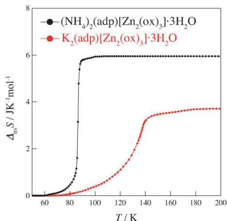
Fig. 4 Transition entropies of  $(\text{NH}_4)_2(\text{adp})[\text{Zn}_2(\text{ox})_3]\cdot 3\text{H}_2\text{O}$  (black) and  $\text{K}_2(\text{adp})[\text{Zn}_2(\text{ox})_3]\cdot 3\text{H}_2\text{O}$  (red).
