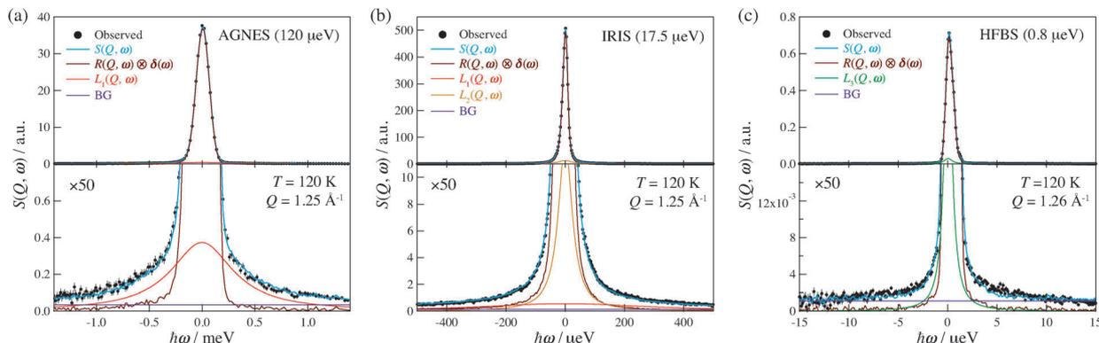
Fig. 7 QENS profiles of  $(\text{NH}_4)_2(\text{adp})[\text{Zn}_2(\text{ox})_3]\cdot 3\text{H}_2\text{O}$  obtained by (a) AGNES, (b) IRIS, and (c) HFBS spectrometers. All data are taken at  $Q \approx 1.25 \text{ \AA}^{-1}$  and  $T = 120 \text{ K}$ . The lower panels display the enlarged plot in the vertical axis. Error bars throughout the text represent one standard deviation. Solid curves represent the results of the fitting analyses. See text for the details.
