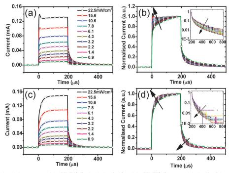
Fig. 2 Transient short-circuit photocurrent of the P3HT/CdSe dot device, (a, b), and the P3HT/CdSe tetrapod device, (c, d), in response to 200 μs square pulsed illumination with a wavelength of 525 nm at various intensities. (a, c) present the raw data while (b,d) present the transient photocurrent curves normalised to the photocurrent value at 200 µs. The insets of figure parts (b) and (d) highlight the decay kinetics of the short-circuit photocurrent transients after normalisation
