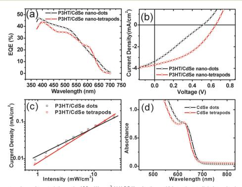
Fig. 1 (a) EQE, (b) current–voltage characteristics under 100 mW cm<sup>-2</sup> AM1.5G illumination and (c) steady state light intensity dependence of the short-circuit photocurrent under monochromatic illumination at 525 nm for the P3HT/CdSe dot (squares) and P3HT/CdSe tetrapod (circles) devices. (d) Absorption spectra of the synthesised CdSe nanoparticles in solution.
