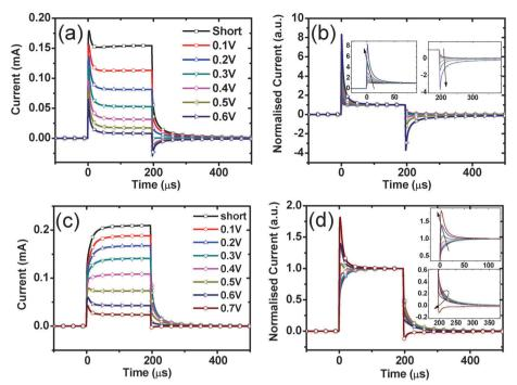
Fig. 3 Transient photocurrent response of the P3HT/CdSe dot (a, b) and P3HT/CdSe tetrapod (c, d) devices to 200  $\mu$ s square-pulse illumination as a function of applied bias voltage. Figure parts (a, c) plot un-normalised traces whereas (b,d) plot normalised traces. Insets of figure parts (b, d) highlight the rise and decay kinetics of the voltage-dependent transients after normalisation. Pulse intensity is  $\sim$  32 mW cm<sup>-2</sup>.
