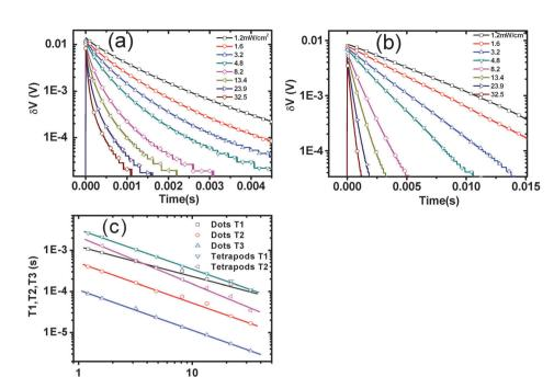
Fig. 6 Photovoltage decay transients plotted as a function of the white background constant illumination intensity for (a) the P3HT/CdSe dot device and (b) the P3HT/CdSe tetrapod device. Data is obtained by plotting the photovoltage transients on a log scale after subtraction of the background voltage. Figure part (c) plots the decay time constants with their linear fit as a function of background light intensity on a log-log scale.
