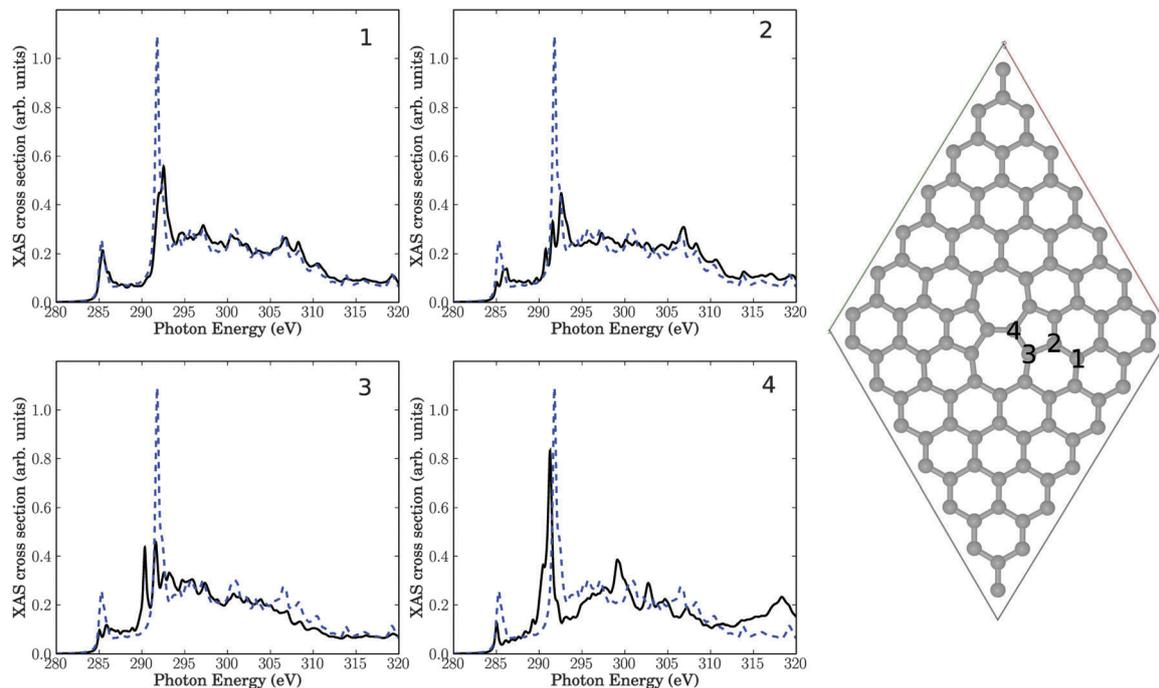
Fig. 3 Right: Stone–Wales (55–77) defect in a  $7 \times 7$  cell. The four panels show NEXAFS spectra corresponding to core-hole creation in atoms 1–4, located close to the defect (see atom numbering). Full, black lines: computed NEXAFS spectra, dashed, blue lines: the theoretical spectrum of unperturbed graphene for comparison.
