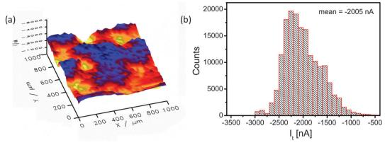
Fig. 5 (a) 3D SECM image of 1000 × 1000 μm<sup>2</sup> region of the ternary oxide based DSA obtained in the sample-generator/tip-collector mode representing the spatial electrocatalytic activity (tip potential  $E_t = 950$  mV; sample potential  $E_s = 1400$  mV vs. Ag/AgCl/3 M KCl). (b) Current distribution histogram extracted from the tip currents of the SECM image in (a).
