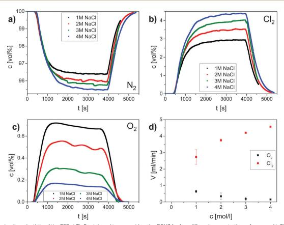
Fig. 2 Monitoring the selectivity of the CER at Ti-Ru-Ir based ternary oxide using DEMS for four different concentrations of agueous NaCl solution. The current density was 400 mA cm $^{-2}$  and the temperature was 25 °C. Example volume fractions of: (a)  $N_2$  (inert gas carrier) (b)  $Cl_2$  (main product) and (c)  $O_2$ (side product); (d) calculated flows in ml min $^{-1}$  for  $Cl_2$  and  $O_2$  as a function of concentration of  $Cl^-$  ions.
