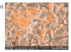
Fig. 4 (a) SEM micrograph of the morphological surface structure of a ternary Ti-Ru-Ir oxide DSA. (b) EDX confirms local Ru enrichment at the electrode surface after electrochemical testing.
