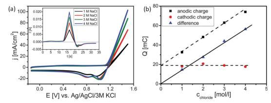
Fig. 3 (a) Cyclic voltammograms of the Ti-Ru-Ir ternary oxide based DSA in 1, 2, 3 and 4 M aqueous solution of NaCl at a scan rate of 100 mV s<sup>-1</sup> and a pH value of 2. The ionic strength was kept constant using NaNO<sub>3</sub>. The inset shows same cyclic voltammogram transformed into the time domain. (b) Charge during the anodic sweep (black cubes), charge during the cathodic sweep (red circles) and the difference charge (blue triangles).
