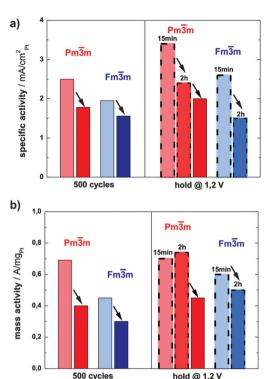
Fig. 4 Comparison of (a) specific and (b) mass activities @ 0.9 V<sub>RHE</sub> of the ordered (red) and the disordered (blue) catalysts after dealloying (500 cycles and potential hold @ 1.2 V for 15 min and 2 hours, respectively) and subsequent degradation (dark red and dark blue color). No subsequent degradation after holding the potential at 1.2  $V_{\text{RHE}}$  was done for the disordered catalyst
