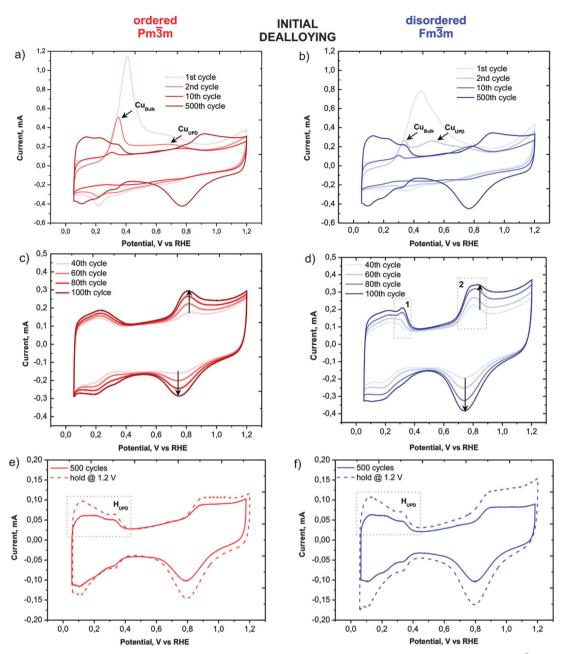
Fig. 3 Selected cyclic voltammograms of the continuously recorded scans during dealloying with 500 cycles of the ordered Pm3m (a, c; red) and the disordered Fm3m (b, d; blue) catalyst, recorded at a scan rate of 0.2 V s<sup>-1</sup>. Comparison of the baseline scans of the ordered (e) and the disordered (f) catalyst after dealloying by cycling (solid line) and potential hold @ 1.2 V for 2 hours (dashed line), recorded at a scan rate 0.05 V s $^{-1}$  in 0.1 M HClO $_4$ .
