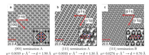
Fig. 4 Simulated STM images of (a) termination A of (001), (b) termination A of (111) and (c) termination B of (111) surfaces obtained using a bias of -2.5 eV. Density ( $\varrho$ ) and tip distance (d) are also indicated. Insets show enlargements of the STM images. In the inset, Fe<sub>A</sub> ions are in grey, Fe<sub>B</sub> ions are in blue and O ions are in red.
