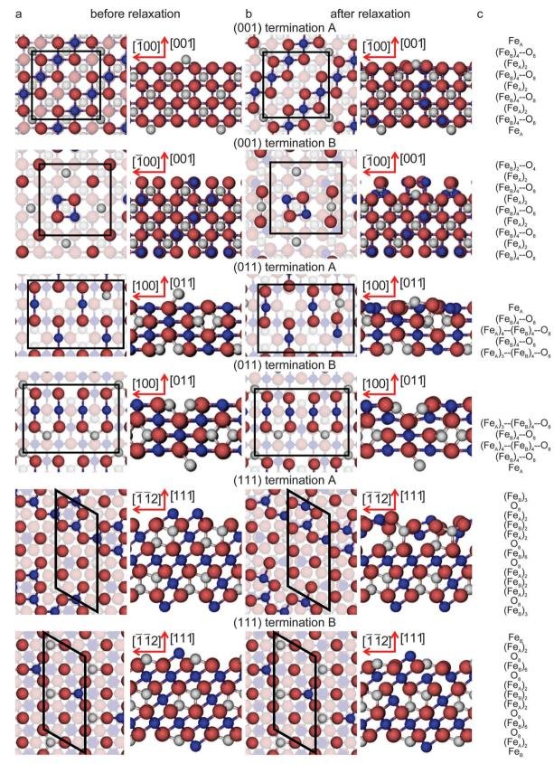
Fig. 2 Top and side view of the simulation slabs for the low-index surfaces of  $Fe_3O_4$ . The surfaces are shown (column a) before, (column b) after relaxation and (column c) their stacking sequence. For the colour code see Fig. 1. Layers with atoms with dangling bonds are highlighted. Crystallographic directions for the top view of (001) surface terminations is [100] for the abscissae towards the right; for the (011) surface terminations it is [011] for the longest axis towards the top.
