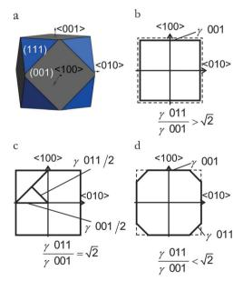
Fig. 3 (a) Equilibrium morphology for a Fe $_3O_4$  crystal derived from a Wulff construction. (b–d) Schemes of the crystal cross-sectional planes along the  $\langle 100 \rangle$  and  $\langle 010 \rangle$  axes for different ratios of stabilities of the lateral surfaces, which illustrate why the (011) surface is absent in the equilibrium morphology.
