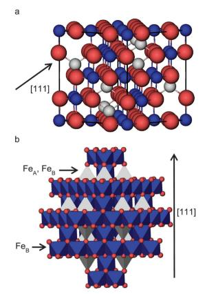
Fig. 1 View of the bulk structure of Fe<sub>3</sub>O<sub>4</sub>: (a) ball and stick model of the cubic unit cell and (b) polyhedral model showing the alternating layers of  $Fe_B$  and  $Fe_A$ – $Fe_B$  ions separated by O ions.  $Fe_A$  ions are in grey,  $Fe_B$  ions are in blue and O ions are in red.
