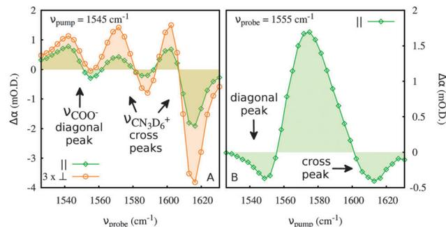
**Fig. 3** (A) Cross section along the probe axis of the 2D-IR spectra for parallel and perpendicular polarization of the pump and probe pulses, and for  $\nu_{\text{pump}} = \nu_{\text{COO}^-}$ . (B) Cross section along the pump axis of the 2D-IR spectrum for parallel polarization of the pump and probe pulses, and for  $\nu_{\text{probe}} = \nu_{\text{COO}^-}$ .
