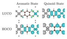
Fig. 7 Electron distribution (at the  $\Gamma$  point) of the HOCO, LUCO for  $Na_{2n}[Ni(C_6H_2S_4)]_n$  (left) and  $[Ni(C_6H_2S_4)]_n$  (right). Note that the HOCO of the aromatic state becomes the LUCO of the oxidized quinoid state. Atoms colour: Ni = bright green, C = brown, S = yellow, H = beige, Na = dark grey
