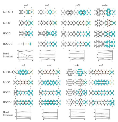
Fig. 4 Electron distribution (at the  $\Gamma$  point) of the HOCO -1, HOCO, LUCO, and LUCO +1, and band structures of the Na<sub>2</sub>(Ni(C<sub>x</sub>S<sub>y</sub>))<sub>n</sub> polymers. The top of the valence band is set to 0, the band energies are in eV, and the Na contribution to the band structures are drawn as dotted lines. Atoms colour: Ni = bright green, C = brown, S = yellow, H = beige, Na = dark grey.
