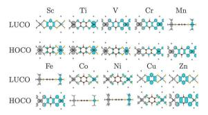
Fig. 9 Electron distribution (at the  $\Gamma$  point) of the HOCO, LUCO as a function of the 3d metal, in octahedral coordination. The results for Sc, Ti, and V are included for completeness, but the oxidation states do not frequently occur in nature. Where the metal  $d_{z^2}$  orbitals are present, a side-on view is used for clarity. Atoms colour: Ni = bright green, C = brown, S = yellow, H = beige, Na = dark grey, N = black spot.
