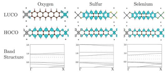
Fig. 5 Electron distribution (at the Γ point) of the HOCO, LUCO and band structures for oxygen, S and Se bridging substituents, respectively. The band energies are given in eV. The Na contribution to the band structures are drawn as dotted lines. Atoms colour: Ni = bright green, C = brown, S = yellow, H = beige, O = red, Se = pea green, Na = dark grey.
