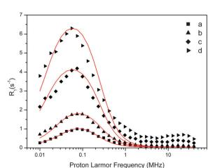
**Fig. 5** Experimental water proton  $R_{1,p}^{\rm OEC}(\omega_{\rm I})$  NMRD difference profiles of OEC (symbols;  $a=29~\mu{\rm M},~b=60~\mu{\rm M},~c=123~\mu{\rm M},~d=188~\mu{\rm M})$  at  $10~^{\circ}{\rm C}$  using theoretical simulation (red line; SBM theory). Parameters are given in Table 2. Note that the peak position is determined by the g-value.
