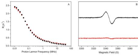
Fig. 3 NMRD profiles (A) and the related EPR spectra (B) of the Mn-depleted Photosystem II (from T. vulcanus) treated by high concentration KCN (black squares and line) and KCl (red circles and line). For the EPR spectra the samples were additionally treated with dithionite to reduce the acceptor side quinone  $Q_A$  to  $Q_A^-$ . NMRD profiles were recorded at 20 °C. EPR spectra were obtained at 13 K; microwave frequency, 9.39 GHz; modulation amplitude, 4 G; microwave power, 200 nW.
