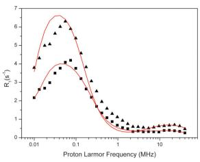
Fig. 7 Fit of the experimental water proton  $R_{1,p}^{\text{QEC}}(\omega_l)$  NMRD difference profiles of the OEC (squares = 123  $\mu$ M, triangles = 188  $\mu$ M) at 10 °C using theoretical simulation (red line) using the slow motion theory and two g-values (g = 4.9 and g = 2.0). Parameters are given in Table 5. Note that the peak positions are determined by the g-values.
