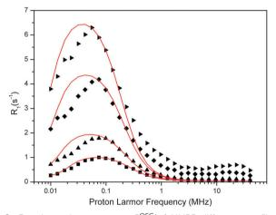
**Fig. 6** Experimental water proton  $R_{\rm LP}^{\rm LC}(\omega_l)$  NMRD difference profiles of OEC (symbols; squares, 29  $\mu$ M; triangles, 60  $\mu$ M; diamonds, 123  $\mu$ M, inverted triangles, 188  $\mu$ M) at 10 °C using theoretical simulation (red line; slow motion theory, eqn (9)). Parameters are given in Table 4. Note that the peak position is determined by the g-value.
