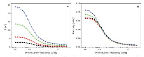
Fig. 1 Panel A displays the proton  $R_1$  NMRD profiles of the intact PSIIcc of T. vulcanus obtained at T = 10 °C for four different PSII reaction center concentrations (29  $\mu$ M, black squares; 60  $\mu$ M, red circles; 123  $\mu$ M, green triangles;  $d = 188 \mu$ M, blue inverted triangles). Panel B displays the same data after normalization to the reaction center concentrations
