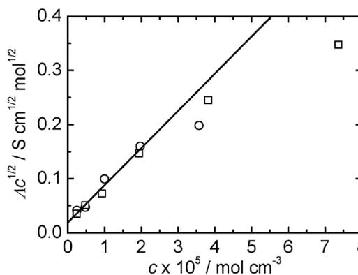
**Fig. 12** Plot of  $A\sqrt{c}$  against  $c$  for the data shown in Fig. 11: ( $\square$ ) [N<sup>n</sup>Bu<sub>4</sub>][B{3,5-C<sub>6</sub>H<sub>3</sub>(CF<sub>3</sub>)<sub>2</sub>}<sub>4</sub>]; and ( $\circ$ ) [NR<sup>f</sup>Bu<sub>3</sub>][B{3,5-C<sub>6</sub>H<sub>3</sub>(CF<sub>3</sub>)<sub>2</sub>}<sub>4</sub>]. The line is the best fit to the low concentration (below  $3 \times 10^{-5}$  mol cm<sup>-3</sup>) data.<sup>34</sup>
