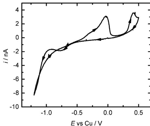
Fig. 18 Cyclic voltammogram for 1.2 mM  $[\text{Cu}(\text{hfac})_2]$  in supercritical  $\text{CO}_2$  with 12.1 wt%  $\text{CH}_3\text{CN}$  containing 20 mM  $[\text{N}^t\text{Bu}_4][\text{BF}_4]$  electrolyte.  $T = 310 \text{ K}$ ,  $p = 17.2 \text{ MPa}$ . The working electrode was a 25  $\mu\text{m}$  diameter platinum disc, the counter electrode was a platinum grid and the reference a 0.5 mm polished copper disc. Sweep rate  $20 \text{ mV s}^{-1}$ .<sup>50</sup>
