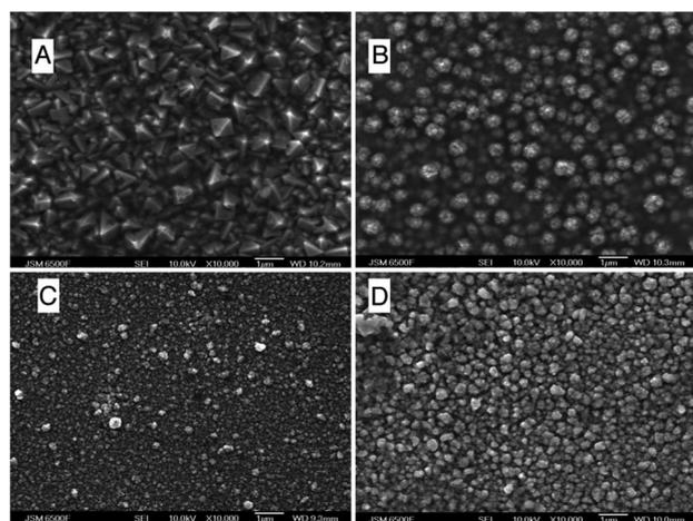
Fig. 17 Electroplated copper SEM images of copper films deposited from a saturated solution of  $[\text{Cu}(\text{CH}_3\text{CN})_4][\text{BF}_4]$  in 87.4 wt%  $\text{CO}_2$ , 12 wt% acetonitrile, 0.6 wt%  $[\text{N}^t\text{Bu}_4][\text{BF}_4]$  309–311 K and 13.8 MPa at (A)  $-0.6 \text{ V}$ , (B)  $-0.9 \text{ V}$ , (C)  $-1.5 \text{ V}$ , and (D)  $-1.7 \text{ V}$  vs. Pt.<sup>5</sup>
