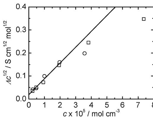
**Fig. 12** Plot of  $A\sqrt{c}$  against  $c$  for the data shown in Fig. 11: ( $\square$ ) [N<sup>n</sup>Bu<sub>4</sub>][B{3,5-C<sub>6</sub>H<sub>3</sub>(CF<sub>3</sub>)<sub>2</sub>]<sub>4</sub>]; and ( $\circ$ ) [NR<sup>fr</sup>Bu<sub>3</sub>][B{3,5-C<sub>6</sub>H<sub>3</sub>(CF<sub>3</sub>)<sub>2</sub>]<sub>4</sub>]. The line is the best fit to the low concentration (below  $3 \times 10^{-5}$  mol cm<sup>-3</sup>) data.<sup>34</sup>
