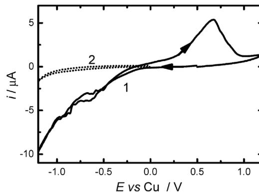
Fig. 19 Scan 1, cyclic voltammogram for 5.3 mM  $[\text{Cu}(\text{hfac})_2]$  in  $\text{scCHF}_3$  with 20 mM  $[\text{N}^t\text{Bu}_4][\text{BF}_4]$  and 0.1 M  $\text{hfacH}$  at 311 K and 17 MPa. Scan 2 shows the background current in the absence of the Cu complex. The working electrode was a 0.37 mm diameter platinum disc, and the counter and reference electrodes were 0.5 mm diameter copper wires. Sweep rate  $100 \text{ mV s}^{-1}$ .<sup>50</sup>
