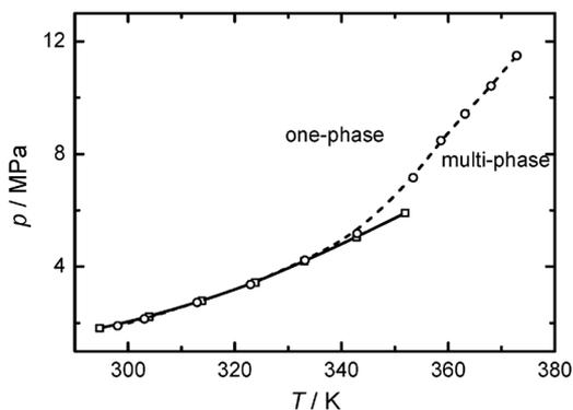
Fig. 20  $p$ - $T$  phase diagrams of the binary mixtures of  $\text{CH}_2\text{F}_2 + \text{A}$ : A =  $\text{GeCl}_4$  ( $\square$ ),  $x_{\text{A}} = 4.4 \times 10^{-3}$ ; and A =  $[\text{N}^t\text{Bu}_4]\text{Cl}$  ( $\circ$ ),  $x_{\text{A}} = 2.95 \times 10^{-3}$ .<sup>6</sup>
