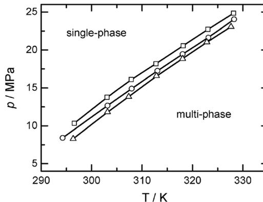
Fig. 10  $p$ - $T$  phase diagram of the mixture  $\text{CO}_2$  (1) +  $\text{CH}_3\text{CN}$  (2) +  $[\text{N}^m\text{Bu}_4][\text{BF}_4](3)$  with and without metal salts (4).  $x_1 = 0.89$ ,  $x_2 = 0.11$  and  $x_3 = 1.34 \times 10^{-5}$ . (○) no metal salt; (△) with  $[\text{Ag}(\text{hfac})(\text{cod})]$ ,  $x_4 = 3.4 \times 10^{-4}$ , and (□) with  $[\text{Cu}(\text{hfac})_2]$ ,  $x_4 = 3.6 \times 10^{-4}$ .<sup>34</sup>
