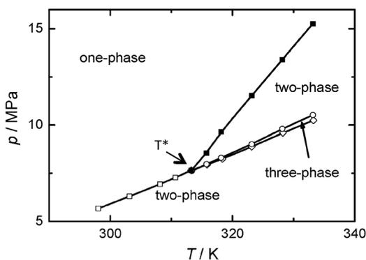
Fig. 9  $p$ - $T$  phase diagram of the mixture of  $\text{CO}_2$  (1) +  $\text{CH}_3\text{CN}$  (2) +  $[\text{N}^m\text{Bu}_4][\text{BF}_4](3)$  with  $x_1 = 0.871$ ,  $x_2 = 0.129$ , and  $x_3 = 8.3 \times 10^{-4}$ . (■) and (□), the phase boundary between one-, and two-phase region; (○) and (◇) mark the region where three phases are in co-existence ( $L_1L_2V$ ). The pressure difference between the two three-phase boundaries is less than 0.3 MPa at 333 K.<sup>34</sup>
