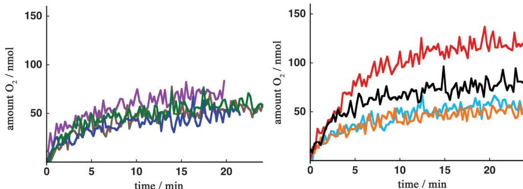
Fig. 2  $O_2$  evolution kinetics by Mn complexes **6** as a function of time. Reaction conditions: an aqueous phosphate buffer solution (0.1 M, pH 7.2, 0.50 mL) containing the Mn complex (20  $\mu$ M) was added to the oxidant  $[Ru(bpy)_3](PF_6)_3$  (3.4 mg, 3.4  $\mu$ mol) and the evolved  $O_2$  was measured in real-time. **6a** (—), **6b** (—), **6c** (—), **6d** (—), **6e** (—), **6f** (—), **6g** (—), **6h** (—).
