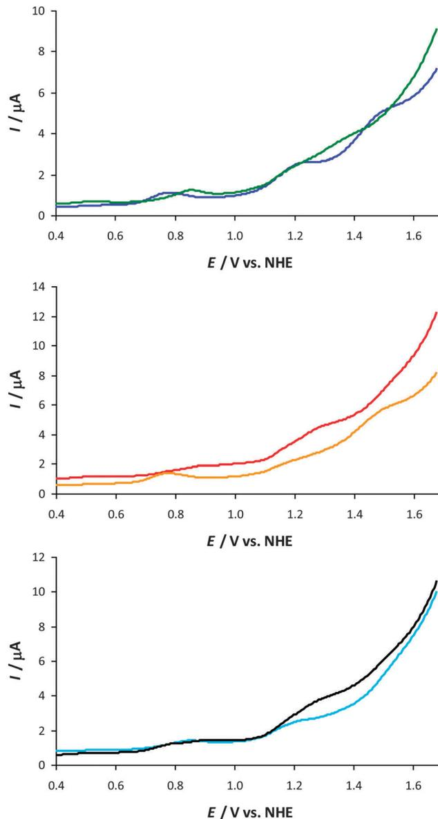
Fig. 5 Differential pulse voltammograms of Mn complexes **6a–b**, **6e–f** and **6g–h** in an aqueous phosphate buffer solution (pH 7.2). Conditions: voltammograms were recorded in an aqueous phosphate buffer solution (0.1 M, pH 7.2) containing the Mn complex (25 μM) with a scan rate of 0.1 V s<sup>-1</sup>. **6a** (—), **6b** (—), **6e** (—), **6f** (—), **6g** (—), **6h** (—).
