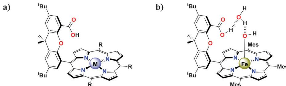
Fig. 6 (a) Structure of a metal "Hangman" porphyrin housing a distal carboxyl group and (b) representation of the hydrogen bonded H<sub>2</sub>O molecule bound between a distal xanthenic carboxylic acid and a Fe porphyrin hydroxide by two hydrogen bonds.
