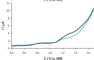
Fig. 5 Differential pulse voltammograms of Mn complexes **6a–b**, **6e–f** and **6g–h** in an aqueous phosphate buffer solution (pH 7.2). Conditions: voltammograms were recorded in an aqueous phosphate buffer solution (0.1 M, pH 7.2) containing the Mn complex (25  $\mu$ M) with a scan rate of 0.1 V s<sup>-1</sup>. **6a** (—), **6b** (—), **6e** (—), **6g** (—), **6h** (—).
