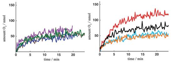
Fig. 2 O<sub>2</sub> evolution kinetics by Mn complexes **6** as a function of time. Reaction conditions: an aqueous phosphate buffer solution (0.1 M, pH 7.2, 0.50 mL) containing the Mn complex (20  $\mu$ M) was added to the oxidant [Ru(bpy)<sub>3</sub>](PF<sub>6</sub>)<sub>3</sub> (3.4 mg, 3.4  $\mu$ mol) and the evolved O<sub>2</sub> was measured in real-time. **6a** (—), 6b (—), 6c (—), 6d (—), 6e (—), 6f (—), 6g (—), 6h (—).
