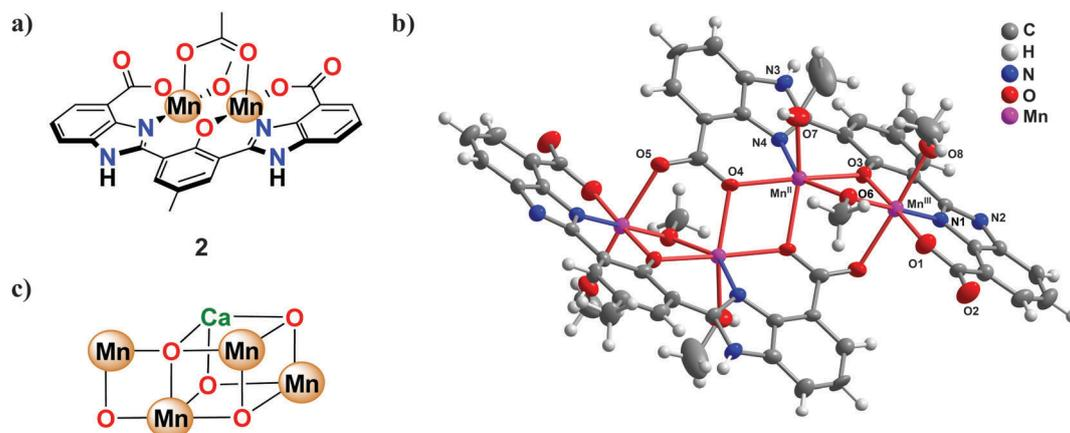
Fig. 1 (a) Molecular structure of the dinuclear Mn<sub>2</sub><sup>II,III</sup> complex **2**, (b) crystal structure of the tetranuclear Mn complex **2'** generated from complex **2**, and (c) representation of the CaMn<sub>4</sub>O<sub>5</sub> active site in the OEC.
