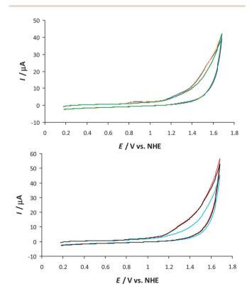
Fig. 4 Cyclic voltammograms of Mn complexes **6a–b,e** and **6f–h** in an aqueous phosphate buffer solution (pH 7.2). Conditions: voltammograms were recorded in an aqueous phosphate buffer solution (0.1 M, pH 7.2) containing the Mn complex (25  $\mu$ M) with a scan rate of 0.1 V s<sup>-1</sup>. **6a** (—), **6b** (—), **6e** (—), **6f** (—), **6g** (—), **6m** (—).
