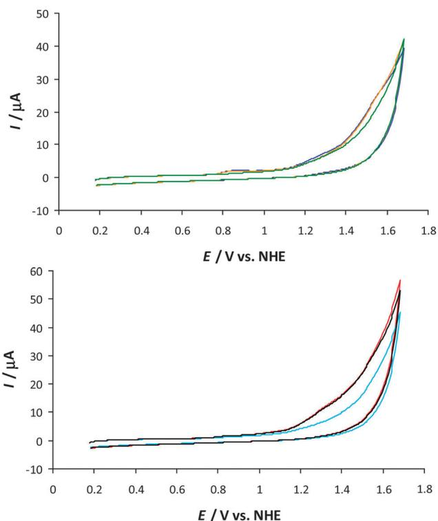
Fig. 4 Cyclic voltammograms of Mn complexes **6a–b,e** and **6f–h** in an aqueous phosphate buffer solution (pH 7.2). Conditions: voltammograms were recorded in an aqueous phosphate buffer solution (0.1 M, pH 7.2) containing the Mn complex (25 μM) with a scan rate of 0.1 V s<sup>-1</sup>. **6a** (—), **6b** (—), **6e** (—), **6f** (—), **6g** (—), **6h** (—).
