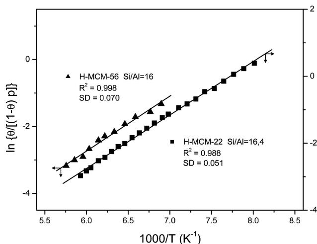
Fig. 11 Plot of the left-hand side of eqn (5) against the reciprocal of the temperature for N<sub>2</sub> adsorbed on H-MCM-22 (Si:Al = 16.4:1) and H-MCM-56; data obtained from the corresponding O–H stretching bands. *R*, linear regression coefficient; SD, standard deviation.
