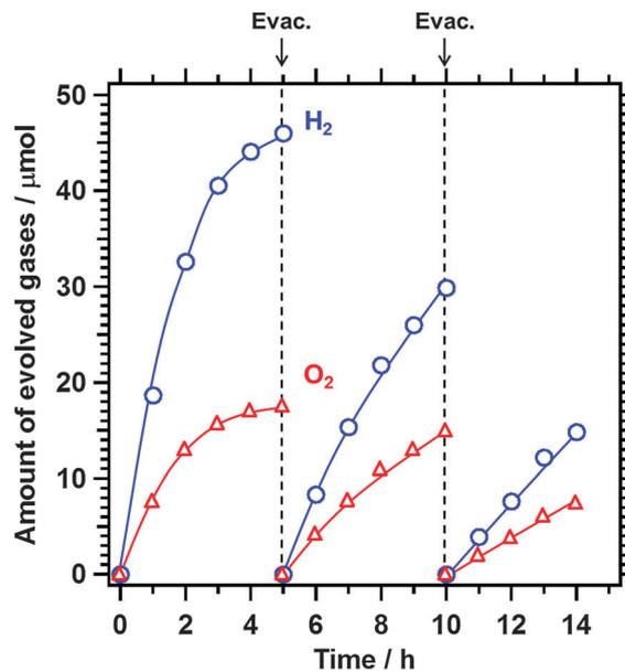
Fig. 6 Time course of Z-scheme water splitting using 2 wt% Pt-loaded  $\text{Sm}_2\text{Ti}_2\text{S}_2\text{O}_5$  ( $\text{S} + \text{HNO}_3$ ),  $\text{TiO}_2$  (rutile), and  $\text{NaI}$  under UV light illumination. Reaction conditions: photocatalysts, 0.2 g each; reaction solution, aqueous  $\text{NaI}$  solution (50 mM, pH = 11, 430 mL); light source: 450 W high-pressure Hg lamp ( $\lambda > 300$  nm).
