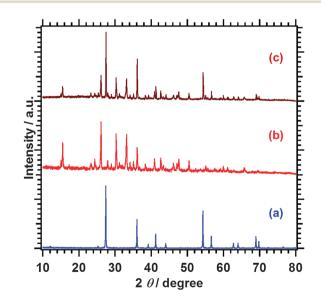
Fig. 7 XRD patterns of (a) rutile-type  $TiO_2$ , (b)  $Sm_2Ti_2S_2O_5$  (S + HNO<sub>3</sub>), and (c) after the Z-scheme water splitting reaction with rutile-type TiO2 at pH 11.
