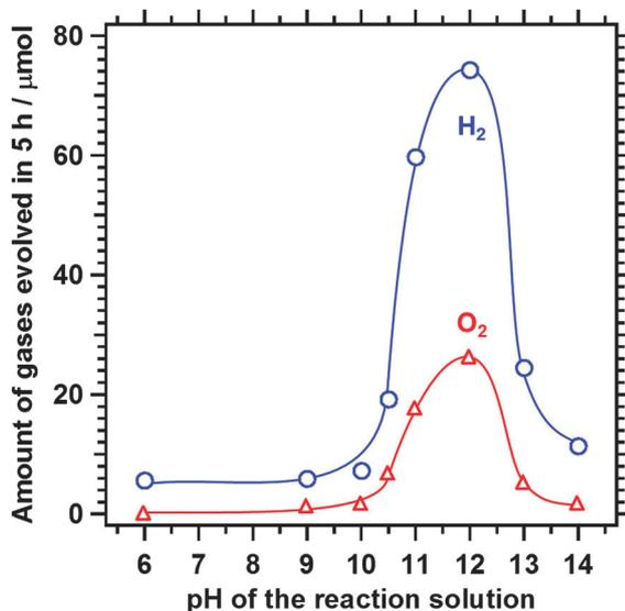
Fig. 5 pH dependence of photocatalytic activity of the Z-scheme system based on 2 wt% Pt-loaded  $\text{Sm}_2\text{Ti}_2\text{S}_2\text{O}_5$  ( $\text{S} + \text{HNO}_3$ ),  $\text{TiO}_2$  (rutile), and  $\text{NaI}$  under UV light illumination. Reaction conditions: photocatalysts, 0.2 g each; solution, aqueous  $\text{NaI}$  solution (50 mM, 430 mL); light source: 450 W high-pressure Hg lamp ( $\lambda > 300$  nm).
