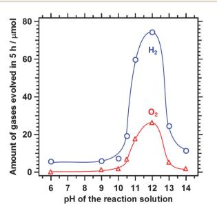
Fig. 5 pH dependence of photocatalytic activity of the Z-scheme system based on 2 wt% Pt-loaded  $Sm_2Ti_2S_2O_5$  (S + HNO3),  $TiO_2$  (rutile), and NaI under UV light illumination. Reaction conditions: photocatalysts, 0.2 g each; solution, aqueous Nal solution (50 mM, 430 mL); light source: 450 W high-pressure Hg lamp ( $\lambda > 300$  nm).
