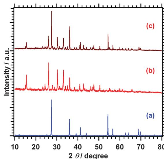
Fig. 7 XRD patterns of (a) rutile-type  $\text{TiO}_2$ , (b)  $\text{Sm}_2\text{Ti}_2\text{S}_2\text{O}_5$  ( $\text{S} + \text{HNO}_3$ ), and (c) after the Z-scheme water splitting reaction with rutile-type  $\text{TiO}_2$  at pH 11.
