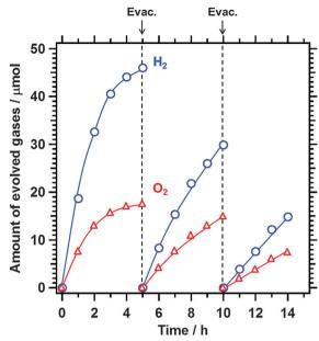
Fig. 6 Time course of Z-scheme water splitting using 2 wt% Pt-loaded Sm<sub>2</sub>Ti<sub>2</sub>S<sub>2</sub>O<sub>5</sub> (S + HNO<sub>3</sub>), TiO<sub>2</sub> (rutile), and NaI under UV light illumination. Reaction conditions: photocatalysts, 0.2 g each; reaction solution, aqueous Nal solution (50 mM, pH = 11, 430 mL); light source: 450 W high-pressure Hg lamp ( $\lambda > 300$  nm).
