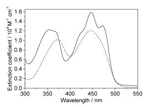
Fig. 2 Experimental data. One-photon absorption spectra of FMN (dashed line) and miniSOG (solid line) in phosphate buffered aqueous solutions.
