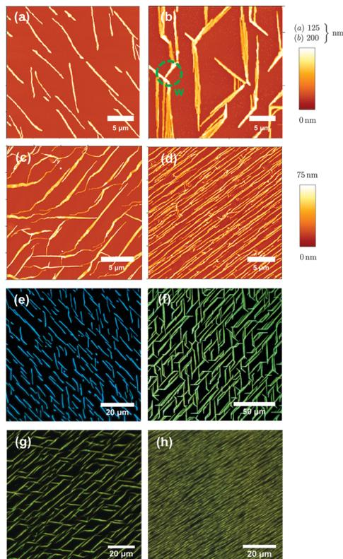
Fig. 3 Same as Fig. 2 but for MONaT, (a, e), MONaT2, (b, f), and MONaT3, (c, d, g, h), deposited at  $T_{\text{sub}} = 377$  K (a, e), 415 K (b, c, f, g), and 360 K (d, h). Nominal thicknesses are  $d = 9$  nm for MONaT, and 18 nm for MONaT2 and MONaT3, respectively; “w” marks a winglet.
