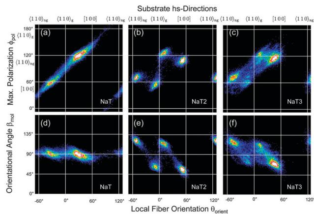
Fig. 6 In the upper panel the correlation between the polarization angle  $\phi_{\text{pol}}$  and the local fiber orientation  $\theta_{\text{orient}}$  is shown. Lines denote substrate hs-directions. The lower panel demonstrates the correlation between the orientational angle  $\beta_{\text{mol}}$  and  $\theta_{\text{orient}}$ .
