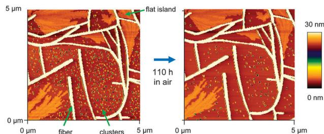
Fig. 5 AFM images of an aging NaT3 sample.
