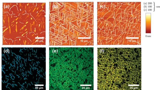
Fig. 2 AFM images (upper panel) and fluorescence microscope images (lower panel) from NaT (a, d), NaT2 (b, e), and NaT3 (c, f). Deposition temperatures are  $T_{\text{sub}} = 360$  K (a, d), and 377 K (b, c, e, f), nominal thicknesses are  $d = 20$  nm, 20 nm, and 10 nm, respectively.
