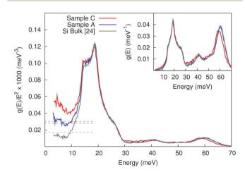
Reduced Density of Phonon States (DPS) for two samples of nanocrystalline Si compared to previously reported results on polycrystalline Si, dotted lines indicate the asymptotic limits from RUS. Inset: DPS.
