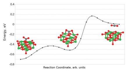
Fig. 10 Reaction profile for an alternative adsorption process, from physisorbed CO<sub>2</sub> to the monodentate chemisorbed species via a tridentate intermediate.
