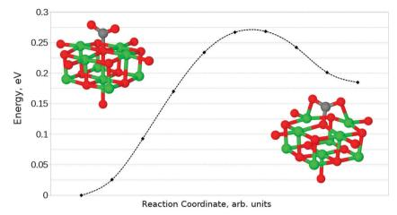
Fig. 8 Reaction profile for the conversion between mono- and tridentate adsorbed CO<sub>2</sub> geometries at an O<sub>50</sub> site obtained using the NEB method with 10 images. A barrier of 0.27 eV (26.05 kJ mol<sup>-1</sup>) is observed for the monodentate-tridentate conversion, while the reverse reaction exhibits a barrier of  $0.09 \text{ eV} (8.68 \text{ kJ mol}^{-1}).$
