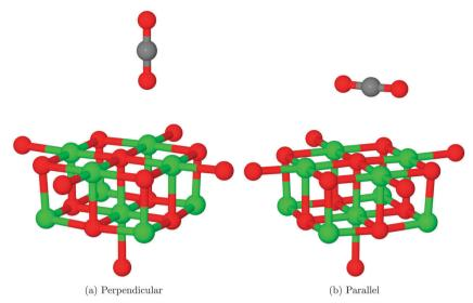
Fig. 5 Physisorption structures identified for CO<sub>2</sub>. In both cases, the oxygen atoms of the adsorbate are coordinated to surface Mg atoms. In the perpendicular case, the  $Mg_s-O_{ads}$  distance for the minimum energy structure was found to be 2.50 Å, while for the parallel structure the two  $Mg_s-O_{ads}$ were equal at 2.76 Å. O atoms shown in red, Mg in green and C in grey.
