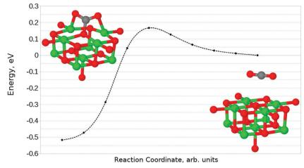
$\textbf{Fig. 9} \quad \text{Reaction profile for the conversion between parallel physisorbed and tridentate adsorbed CO$_2$ geometries on the defect-free MgO(100) terrace$ obtained using the NEB method with 10 images. A barrier of 0.17 eV (17.40 kJ mol<sup>-1</sup>) is observed for the adsorption process.
