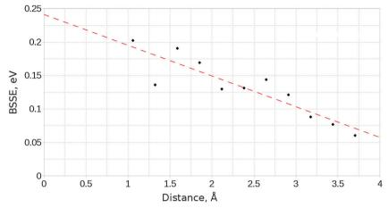
Fig. 2 Variation of the basis-set superposition error with the distance between surface and adsorbate components for the unmodified MgO surface and a parallel orientated CO2 molecule.
