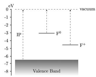
Fig. 4 Positions of defect levels of MgO and their vertical ionization potentials. MgO (100) terrace IP: 6.46 eV, F<sup>0</sup>: 3.05 eV, F<sup>+</sup>: 4.55 eV. Relaxation to the ground states corresponding to MgO+, F+ and F2+ gave values for the adiabatic ionization potentials of 5.52, 1.91 and 3.30 eV respectively.
