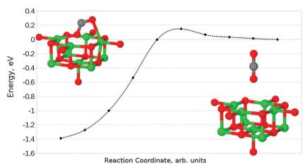
Fig. 15 Reaction profile for the perpendicular adsorption of CO<sub>2</sub> at an F<sup>+</sup> centre on the MgO(100) terrace, obtained using the NEB method with 10 images. Counterpoise corrections not included
