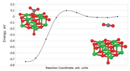
Reaction profile for the adsorption of  $CO_2$  at an  $O_{5c}$  site obtained using the NEB method with 10 images. Counterpoise corrections not included.
