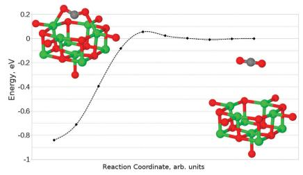
Fig. 14 Reaction profile for the parallel adsorption of CO<sub>2</sub> at an F<sup>+</sup> centre on the MgO(100) terrace, obtained using the NEB method with 10 images. Counterpoise corrections not included
