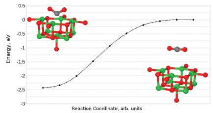
Fig. 12 Reaction profile for the perpendicular adsorption of CO<sub>2</sub> at an F<sup>0</sup> centre on the MgO(100) terrace, obtained using the NEB method with 10 images. No barrier to adsorption is observed. Counterpoise corrections not included
