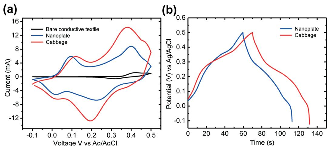
Fig. 5 (a) Cyclic voltammetry curves and (b) galvanic charge-discharge plots of the nanoplates and cabbage-like  $\beta$ -Co(OH)<sub>2</sub> nanostructures on the conductive textile substrate.
