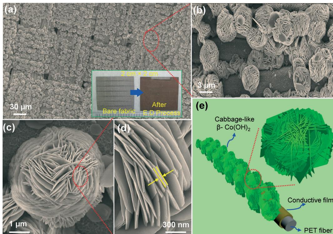
Fig. 1 FE-SEM images of the cabbage-like  $\beta$ -Co(OH) $_2$  nanostructures on the conductive textile substrate synthesized at an external applied voltage of  $-0.75$  V for 4 h: (a) perspective view and (b–d) high-magnification views. (e) 3D schematic diagram of the corresponding structures. The inset of (a) shows the photographic images of the conductive textile fabric before and after ED.
