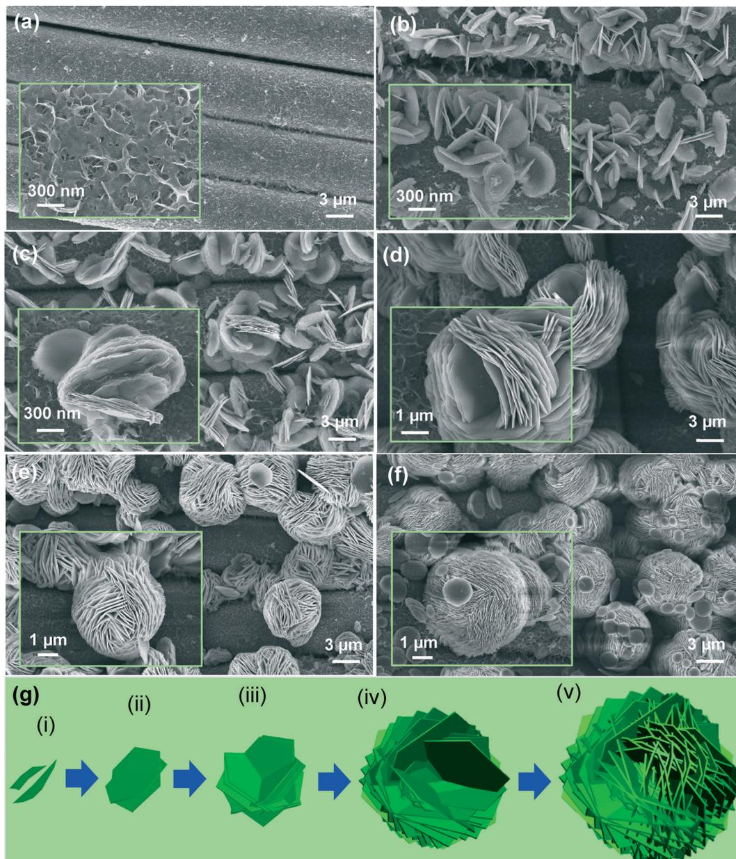
**Fig. 2** FE-SEM images of the cabbage-like  $\beta$ -Co(OH) $_2$  nanostructures on the conductive textile at different growth times of (a) 30 min, (b) 1 h, (c) 1.5 h (d) 2 h (e) 4 h, and (f) 8 h under the constant external applied voltage of  $-0.75$  V. (g) Schematic illustration of the structural formation of the cabbage-like  $\beta$ -Co(OH) $_2$  nanostructures.
