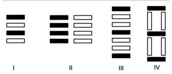
Fig. 1 Schematic representations of structural types I-IV. The black and white rectangles represent donor and acceptor groups respectively.
