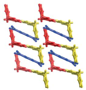
Fig. 4 A stick representation of  $[(4)_2F_4TCNQ]$  showing the formation of "channels" by elbow-shaped cations (red and gold) and the location of  $F_4 TCNQ^{2-}$  anions (blue) within the channels. The channels extend into the page.
