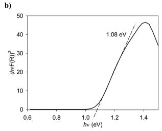
Fig. 9 a) The Vis-NIR solid-state diffuse reflectance spectrum of  $[(1)F_4TCNQ]$ . b) The Tauc plot derived from the spectrum showing the estimation of the optical band gap.
