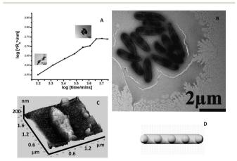
Fig. 5 a) Ripening of the [PMo<sub>12</sub>] spheres in a sonicated dispersion into peapods with time. b) TEM image of the peapods. c) AFM image of a peapod. d) A model of a peapod.
