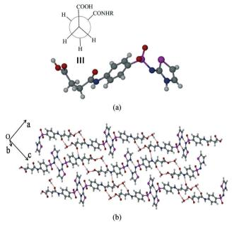
Fig. 3 SST/monohydrate (SST/H2O). (a) Syn geometry adopted at -CH<sub>2</sub>-CH<sub>2</sub>- group of SST. (b) Packing of two adjacent chains, showing the interactions formed by bridging water molecules between two SST molecules.
