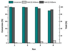
Fig. 5 Recycling experiment of the hydrogenation of diphenylacetylene over Ni-0.5@CNTs at 50 °C, 5 bar H<sub>2</sub> for 7 h.
