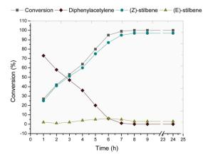
Fig. 4 Evolution in time of diphenylacetylene semi-hydrogenation in the presence of Ni-0.5@CNTs at 50  $^{\circ}$ C, 5 bar H<sub>2</sub> for 24 h.
