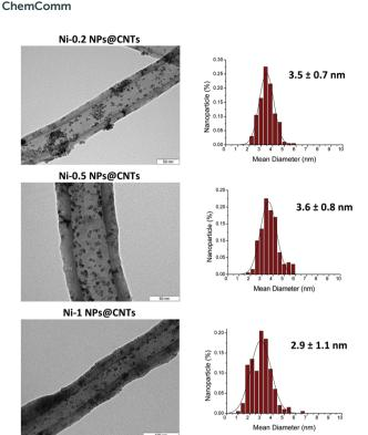
Fig. 2 TEM micrographs and size distributions of supported Ni-0.2, Ni-0.5 and Ni-1 NPs@CNTs.
