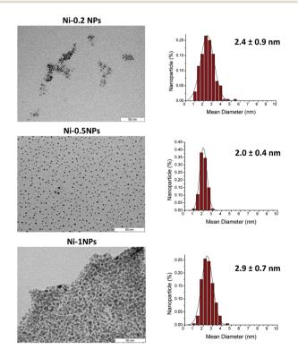
Fig. 1 TEM micrographs and size distributions of Ni-0.2, Ni-0.5 and Ni-1
