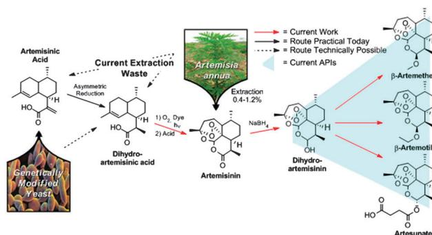
Fig. 1 Overall production scheme of anti-malaria APIs from artemisinin obtained by traditional extraction from *Artemisia annua* and genetically modified yeast combined with chemical modification. Dihydroartemisinin (4), combined with piperazine in Eurartesim, Artekin and Duo-Cotecxin),  $\beta$ -artemether (5, combined with lumefantrine in Coartem),  $\beta$ -arteether (6, Artemotil), and  $\alpha$ -artesunate (7, combined with amodiaquine in Coarsucam and ASAQ-Winthrop).
