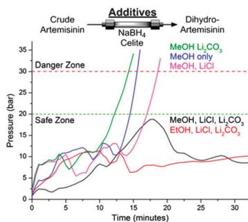
Fig. 2 System pressure observed during reduction of crude artemisinin **3** as a function of cosolvent and solid additives in the Celite<sup>®</sup>/NaBH<sub>4</sub> column.
