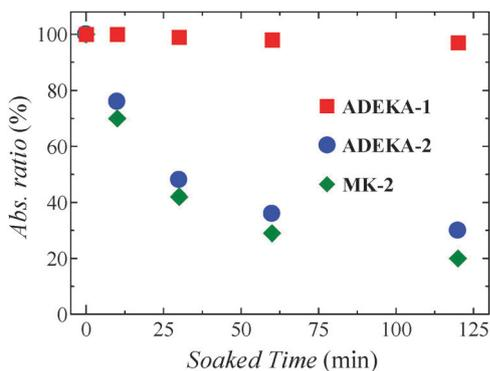
Fig. 2 Changes of the absorbances due to the carbazole dyes (**ADEKA-1**, **ADEKA-2** and **MK-2**) adsorbed on the TiO<sub>2</sub> electrodes with the soaked time into 3-methoxypropionitrile–water (1 : 1 in volume) at 85 °C in the dark.
