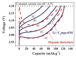
Fig. 5 Charge cycles of an equimolar mixture of [Li][FSI] and  $[C_3mpyr][FSI]$  in a Li|LiCoO<sub>2</sub> cell; dashed lines = organic electrolyte, solid lines = the Li<sup>+</sup>/[C<sub>3</sub>mpyr][FSI] electrolyte. Redrawn from ref. 112.
