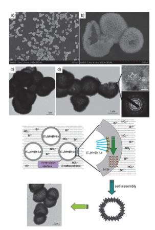
Fig. 14 SEM and HRTEM images of BiOBr HMSs (top) and a plausible schematic formation process of the BiOBr HMSs (bottom). Reproduced from ref. 181 with permission from Wiley-VCH.
