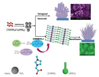
Fig. 13 Schematic illustration for the growth process of TiO<sub>2</sub>. Reproduced from ref. 180 with permission from the RSC.
