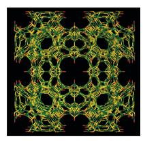
Fig. 6 A [001] perspective view of the framework structure of aluminophosphate molecular sieve DNL-1 (Al yellow, P green, and O red). The bridging oxygen atoms in the framework and all hydrogen atoms have been omitted for clarity. Reproduced from ref. 144 with permission from Wilev-VCH
