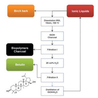
Scaled up betulin isolation process (MW: microwave heating).<sup>214</sup>
