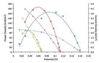
Fig. 4 Power vs. potential (solid line) and current vs. potential (dotted line) plots from thermoelectrochemical devices utilizing platinum electrodes and 0.1 M  $\text{Co}^{\text{II/III}}(\text{bpy})_3(\text{NTf}_2)_{2/3}$  in  $[\text{C}_2\text{mim}][\text{B}(\text{CN})_4]$  at three temperature differences:  $T_{\text{hot}}$  (°C)/ $T_{\text{cold}}$  (°C): 130/30 (blue); 130/60 (red); 130/90 (green). Reproduced from ref. 85 with permission of the RSC.
