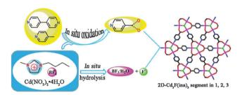
Fig. 9 The formation routes of F-centered Cd<sub>3</sub>F MOFs via in situ oxidation and hydrolysis. Reproduced from ref. 153 with permission from the RSC.
