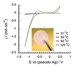
Fig. 3 The appearance of the acid-containing plastic crystal supported on cellulose acetate membrane, and the cyclic voltammogram for 4% HNTf<sub>2</sub> + [Chol][H<sub>2</sub>PO<sub>4</sub>] membrane. Reproduced from ref. 67 with permission from Elsevier
