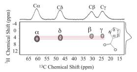
Fig. 1 <sup>2</sup>H-<sup>13</sup>C HETCOR MAS spectrum for U-[<sup>2</sup>H<sub>7</sub>, <sup>13</sup>C<sub>5</sub>, <sup>15</sup>N]-Pro labelled A. aurantia dragline silk. Rotor-synchronized sampling in the indirect dimension was used to eliminate spinning sidebands and obtain a narrow spectral-width high-resolution spectrum. The  $^2\mathrm{H}^{-13}\mathrm{C}$  correlation is indicated for each Pro site in the spectrum (red lines).
