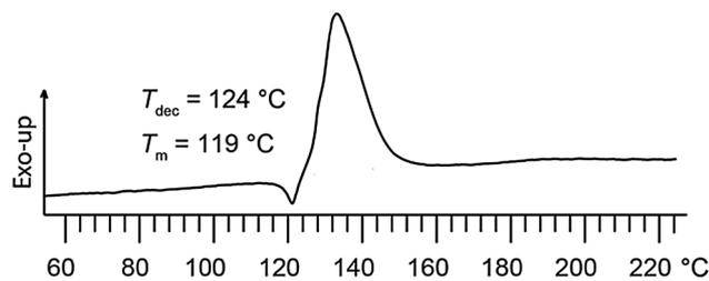
Fig. 1 DSC plot of TNM<sub>2</sub>-BOD (**2**), recorded with a heating rate of 5 °C min<sup>-1</sup>.
