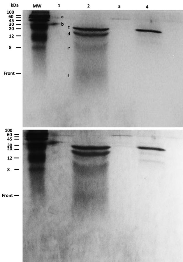
**Fig. 9** SDS-PAGE assay run for 15% polyacrylamide gel stained with Coomassie R (upper) or G250 (lower panel). Bands were detected on lane 1(a–b), 2(c–d and f), 3(a–c) and 4 (a–e). Lane 1: 1.5 wt%  $KA_6E$ , Lane 2: 1.5 wt%  $KA_6E$  + 0.026 wt% elastase ( $M_{rE} = 2129$ ), Lane 3: 0.0062 wt%  $KA_6E$  + 0.00011 wt% elastase ( $M_{rE} = 2080$ ), Lane 4: 0.13 wt% elastase.
