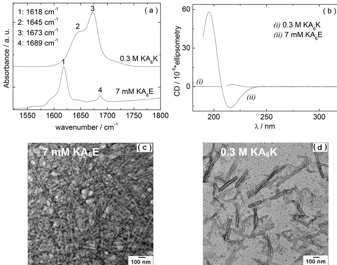
Fig. 1 (a) FTIR spectra, (b) CD spectra (obtained on a Chirascan spectrometer), and (c–d) TEM data obtained for 7 mM  $\text{KA}_6\text{E}$  and 0.3 M  $\text{KA}_6\text{K}$  solutions in water. FTIR data for  $\text{KA}_6\text{K}$  in (a) has been shifted in order to enable the visualization of the data.
