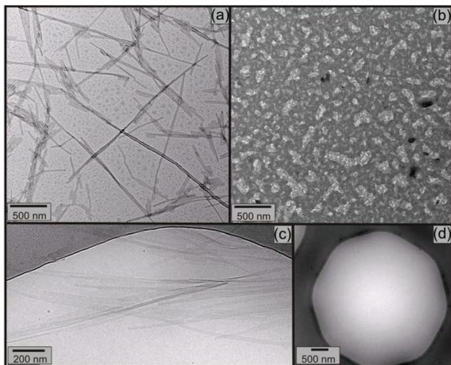
**Fig. 7** TEM images obtained for samples dried from (a) 7 mM KA<sub>6</sub>E and (b) 7 mM KA<sub>6</sub>E; Mr<sub>E</sub> = 2.3 × 10<sup>3</sup> solutions in Trizma pH 8. Cryo-TEM images measured for (c) 14 mM KA<sub>6</sub>E and (d) 14 mM KA<sub>6</sub>E; Mr<sub>E</sub> = 2.3 × 10<sup>3</sup> solutions in Trizma pH 8.
