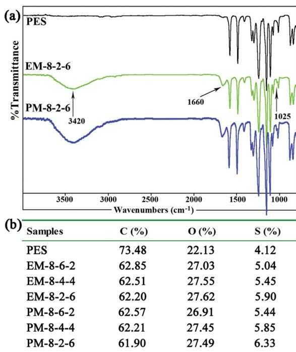
Fig. 2 (a) FTIR spectra of the PES and the modified PES membranes; (b) the contents of the elements C, O, and S in the modified membranes detected by XPS (mass fraction).
