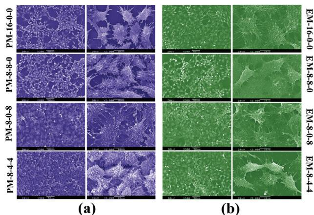
Fig. 10 SEM pictures of human hepatocytes LO2 cultured on the membranes for 2 days: (a) hepatocytes on phase-inversion membranes; (b) hepatocytes on evaporation membranes.
