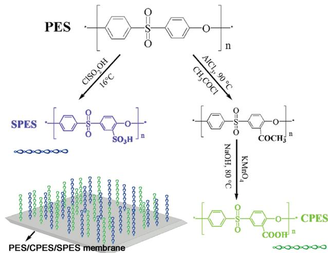
**Scheme 1** Synthetic procedure for the SPES and CPES polymers. The PES/CPES/SPES composite membranes were prepared by blending SPES, CPES, and PES at different ratios with surface aggregated functional sulfonic acid and carboxylic acid polymer chains.
