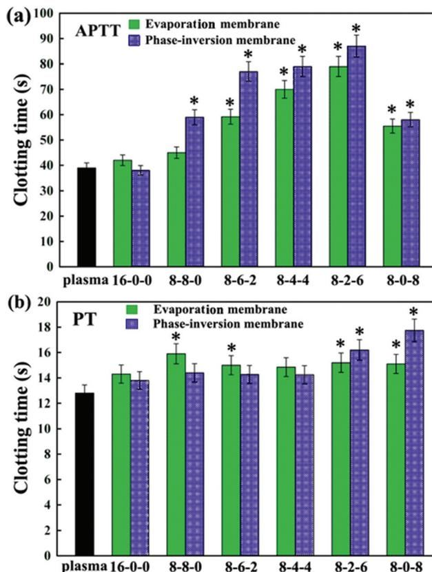
Fig. 7 (a) APTT, and (b) PT assays for the PES and modified PES membranes. The results are expressed as means  $\pm$  SD ( $n = 3$ ), \* $P < 0.05$  compared to the values of the 16-0-0 membrane (APTT and PT).
