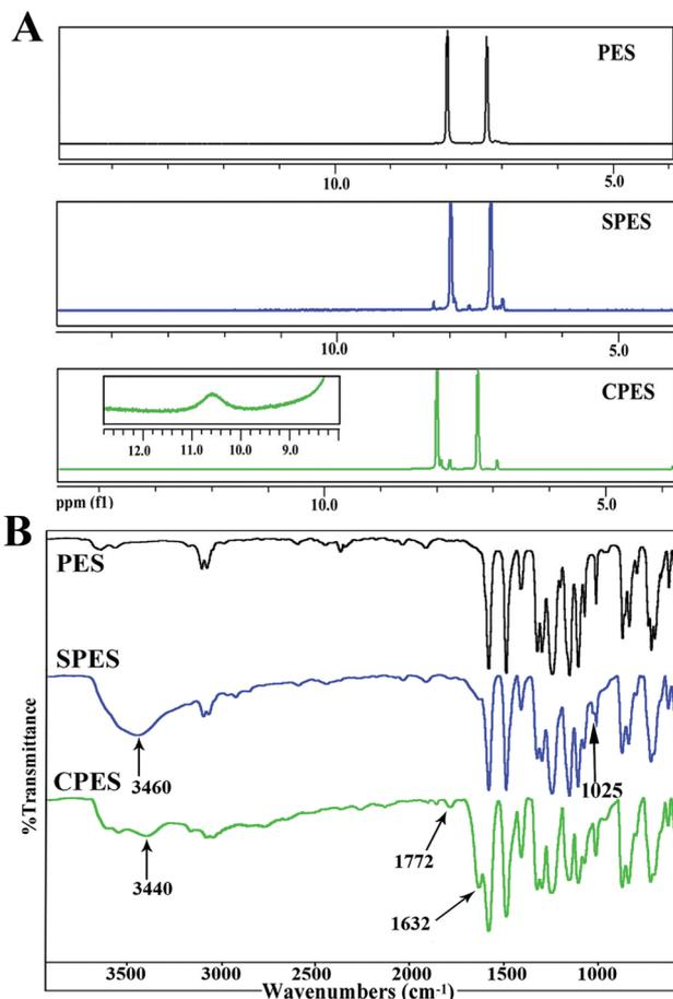
Fig. 1 (A) <sup>1</sup>H-NMR spectra of SPES and CPES. For CPES, the inserted figure of chemical shift at 9–12 ppm was obtained by amplifying the baseline; (B) FTIR spectra of SPES and CPES.
