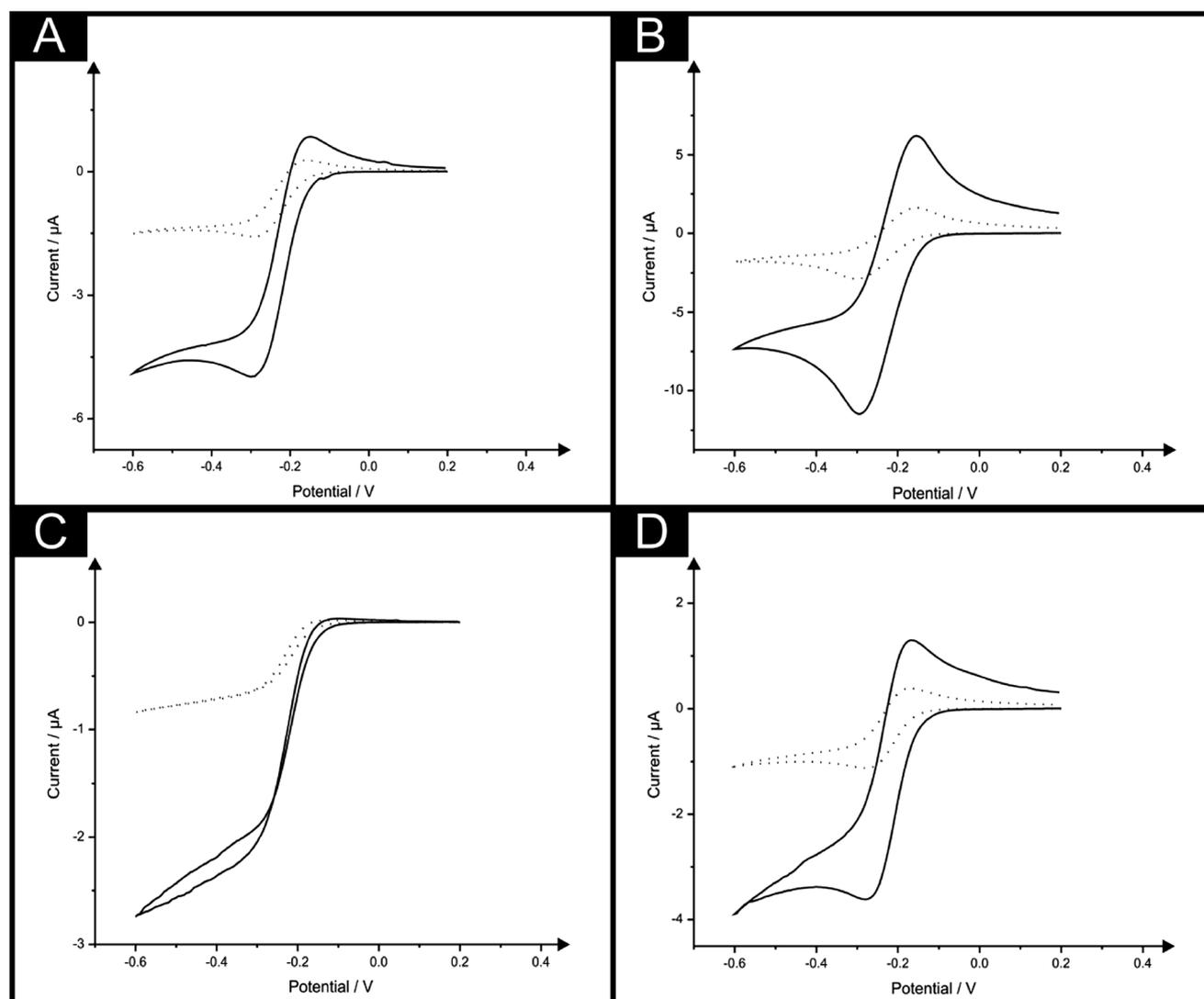
Fig. 4 Cyclic voltammograms recorded in 1 mM hexaammine-ruthenium(III) chloride/0.1 M KCl using a single B-SPE (dotted line) and  $\text{B}^4\text{-SPE}$  (solid line) at scan rates of 5  $\text{mV s}^{-1}$  (A) and 100  $\text{mV s}^{-1}$  (B). Also shown are cyclic voltammograms obtained using a single  $\mu\text{B-SPE}$  (dotted line) and  $\mu\text{B}^4\text{-SPE}$  (solid line) at scan rates of 5  $\text{mV s}^{-1}$  (C) and 100  $\text{mV s}^{-1}$  (D).
