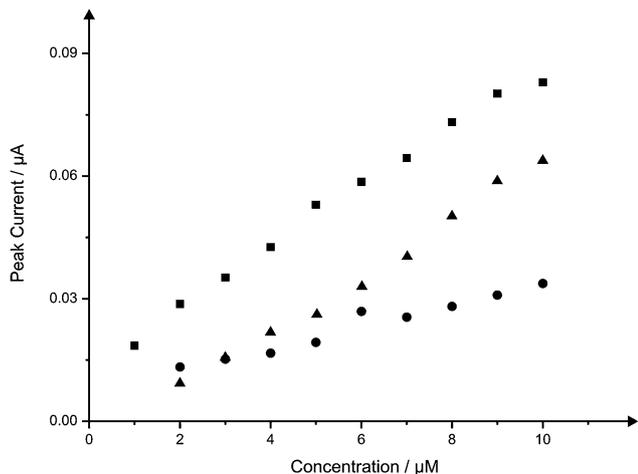
Fig. 6 Calibration plots resulting from the addition of NADH (1 to 10  $\mu\text{M}$ ) into a pH 7 phosphate buffer solution using the B-SPE (circles) and B<sup>2</sup>-SPE (squares) at a scan rate of 50  $\text{mV s}^{-1}$  and B-SPE (triangles) at a scan rate of 200  $\text{mV s}^{-1}$ .
