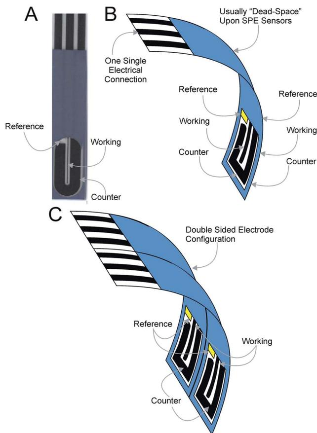
Fig. 2 (A) An optical image of a typical B<sup>2</sup>-SPE showing the electrode layout of the working, counter and reference electrodes. (B) and (C) depict conceptual images introducing the B<sup>2</sup>-SPE and B<sup>4</sup>-SPEs respectively where in this configuration the electrodes are fabricated back-to-back and share a common set of electrical connections to the potentiostat.
