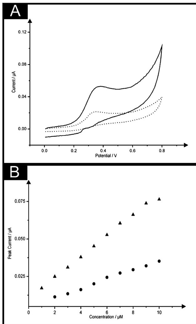
Fig. 5 (A) A comparison of cyclic voltammograms obtained in 6  $\mu$ M NADH in a pH 7 phosphate buffer solution using the B-SPE (dotted line) and B<sup>2</sup>-SPE (solid line). Scan rate: 50 mV s<sup>-1</sup>. (B) Overlaid calibration plots for the addition of NADH (1 to 10  $\mu$ M) into a pH 7 phosphate buffer solution at the B-SPE (circles) and B<sup>2</sup>-SPE (triangles).
