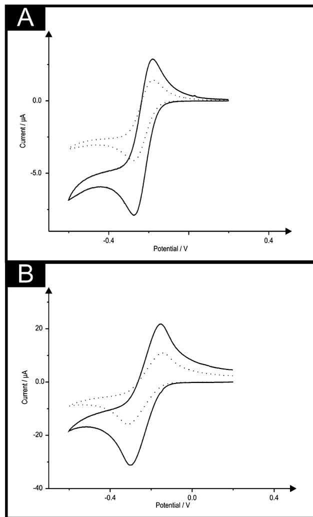
Fig. 3 Cyclic voltammograms recorded in 1 mM hexaammine-ruthenium(III) chloride/0.1 M KCl at scan rates of 5 mV s<sup>-1</sup> (A) and 100 mV s<sup>-1</sup> (B) using a single ST-SPE (dotted line) and ST<sup>2</sup>-SPE (solid line).
