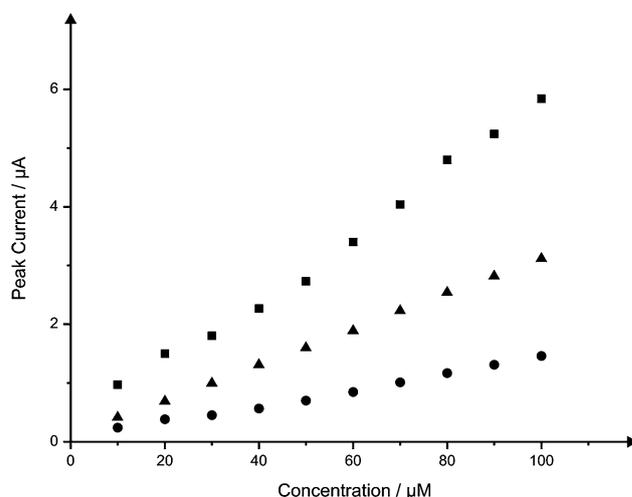
Fig. 7 Overlaid calibration plots for the addition of nitrite (10 to 100  $\mu\text{M}$ ) into a pH 7 phosphate buffer solution at the B-SPE (circles) and B<sup>2</sup>-SPE (triangles) and B<sup>4</sup>-SPE (squares). Cyclic voltammograms corresponding to the response obtained at the three electrode configurations at a concentration of 60  $\mu\text{M}$  nitrite are shown in ESI Fig. 6.†
