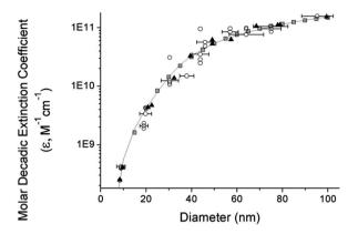
Fig. 5 Molar decadic extinction coefficient ( $\varepsilon$ ) for silver nanoparticles. Data obtained experimentally (empty circles, selected points show the x-error as size S.D. determined from HR-TEM), obtained from manufacturer supplied information (black triangle), and simulated data (grey squares).
