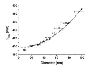
**Fig. 4** Absorbance peaks for silver nanoparticles obtained experimentally (empty circles), manufacturer supplied information (black triangles) and simulated (empty squares). The *x*-error is the S.D. of the diameter.
