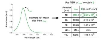
Scheme 1 Calculation of the silver nanoparticle concentration. The extinction coefficient of citrate-coated nanoparticles can be calculated using Table S1† and the diameter of the nanoparticles estimated by  $\lambda_{\text{max}}$  or by TEM.
