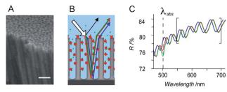
Fig. 2 (A) SEM image of the AAO chip (scale bar: 500 nm). (B) Scheme of the sensing concept. Avidin (red dots) adsorbs on the pore walls of the AAO chip and causes a red shift of the interference spectrum as shown in (C) (blue and red curves). When the dye-labelled biotin (green dots leading to the green beam) binds to the immobilised avidin, the reflectivity of the system is attenuated at the absorption maximum of the Atto dye, which is shown as a drop in the spectrum in (C) (the green curve)
