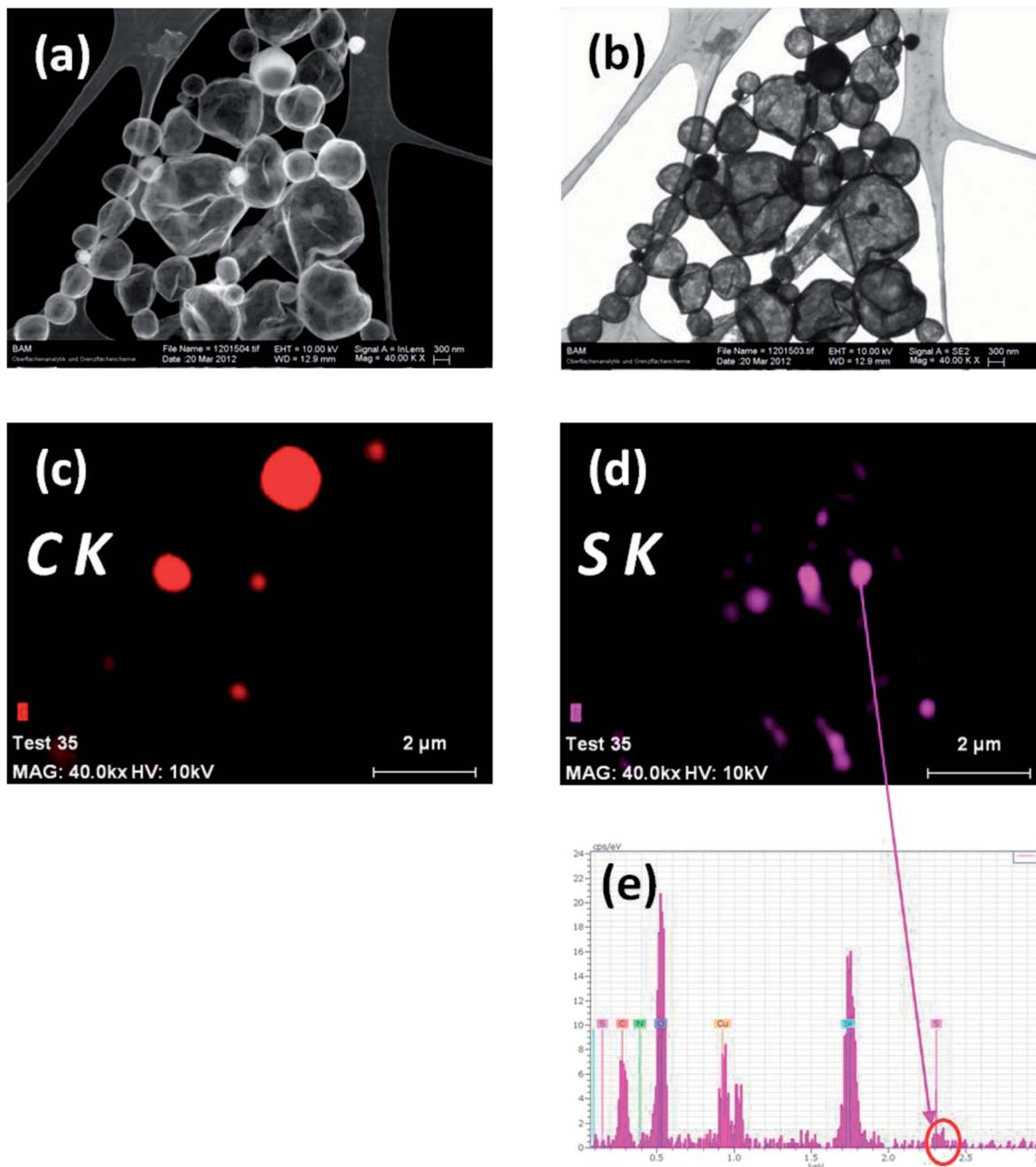
Fig. 6 Upper (a) and in-transmission (b) SEM observation of  $\text{SiO}_2$  submicrocapsules prepared on lacey carbon foils. EDX elemental maps of C K (c) and S K in the range of the detection limit (d) with the corresponding X-ray spectrum (e) from the marked area.
