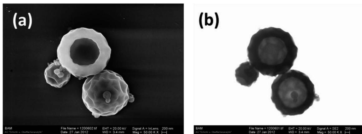
Fig. 3 Example of complementary “upper” observation of polyepoxide-shell and oil-core particles submicrocapsules using the *In-Lens* detector (a) and in the transmission mode (b). Note the details on the outer particle surface as well as the presence of many nanoparticles in the left micrograph and the quite different occurrence of the big, bottom particle in the two imaging modes.
