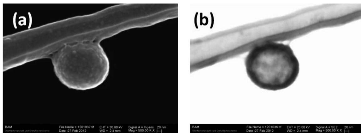
Fig. 2 Example of complementary “upper” observation of a single SiO<sub>2</sub> submicrocapsule (about 200 nm size) onto a string of the supporting lacey carbon foil using the *In-Lens* detector (a) and in the transmission mode (b). Note the “shell-like” structure of the particle that can be visualized only in the transmission mode.
