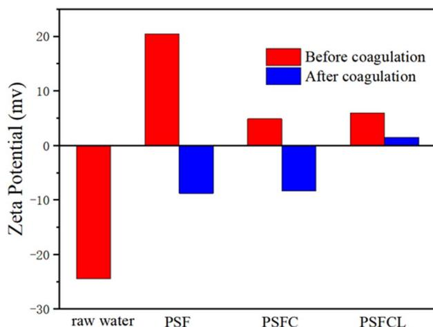
Fig. 6 Zeta potential of raw water, PSF, PSFC, PSFCL before and after coagulation.
