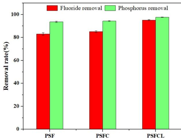
Fig. 4 Comparison of removal efficiency of three flocculants under optimized conditions (La/Si molar ratio = 0.3, pH = 5, dosage = 30 ml L<sup>-1</sup>, agitation time = 10 h, sedimentation time = 30 min).
