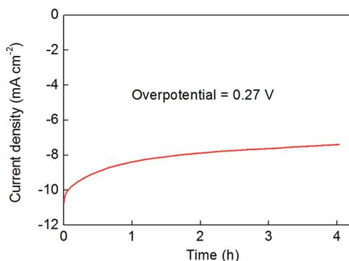
**Fig. 6** Controlled potential bulk electrolysis of a 300 nm-thick Co<sub>2</sub>Mo<sub>9</sub>S<sub>26</sub> film on an FTO support at a fixed, resistance-corrected overpotential for the hydrogen evolution reaction of 270 mV. The electrolyte was 0.5 M H<sub>2</sub>SO<sub>4</sub> and was stirred throughout (see Experimental section for further details).
