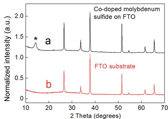
Fig. 1 (a) XRD pattern of a Co-doped molybdenum sulfide film grown on an FTO substrate (black). The peak associated with the hexagonal structure of  $\text{MoS}_2$  is highlighted with the asterisk. (b) The XRD pattern of a blank FTO substrate for comparison (red).
