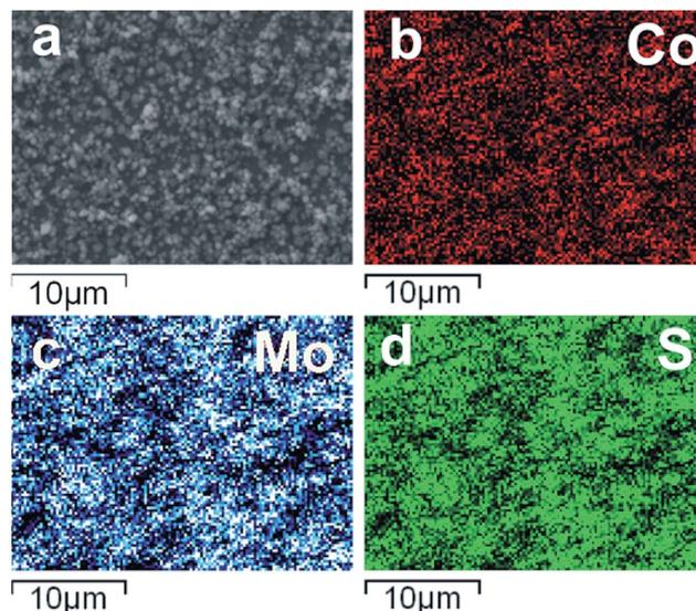
Fig. 3 SEM images and the corresponding elemental mapping for Co, Mo and S in a  $\text{Co}_2\text{Mo}_9\text{S}_{26}$  film, indicating the homogeneous distribution of Co atoms within the sample.
