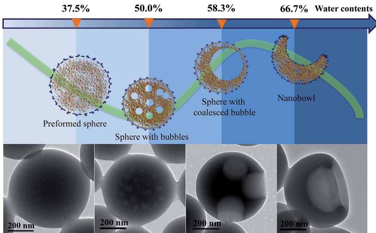
Fig. 5 Evolution of nanobowls from PHAzoMA<sub>226</sub>. With the addition of water, PHAzoMA<sub>226</sub> forms preformed spheres, spheres with bubbles, spheres with coalesced bubbles and nanobowls at different water contents. The TEM images show the corresponding nanostructures at the various water contents from left to right.
