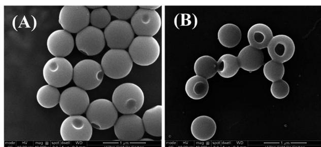
Fig. 2 SEM images of nanobowls formed from (A) PHAZoMA<sub>29</sub> and (B) PHAZoMA<sub>116</sub>.
